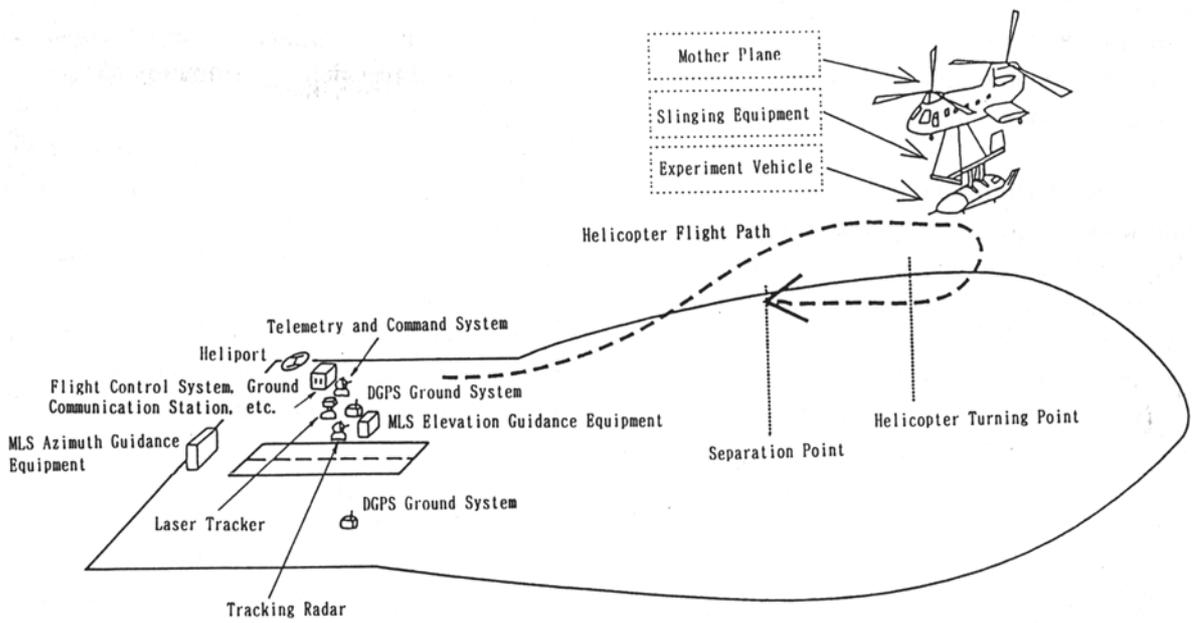
Fig. 6 Conceptual Drawing of Experimental System
