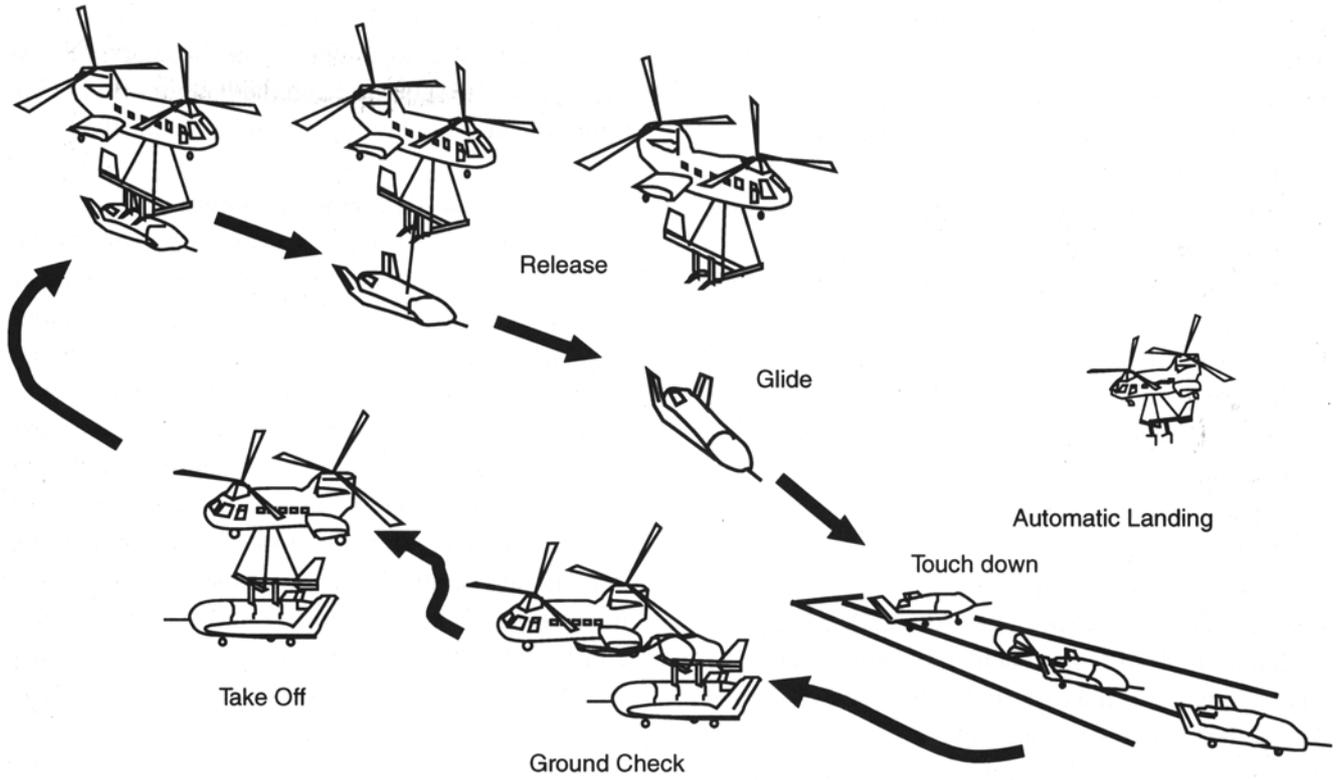
Fig. 3 Sequence of Automatic Landing Flight Experiment
