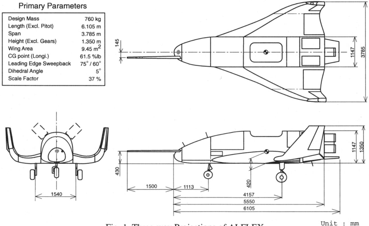
Fig. 1 Three-way Projections of ALFLEX
