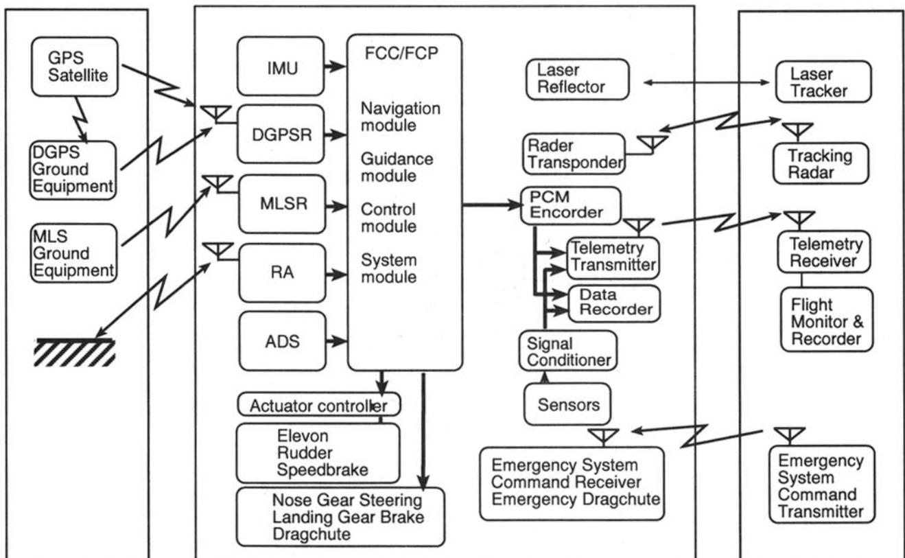
Fig. 5 Schematic Diagram of Experiment System
