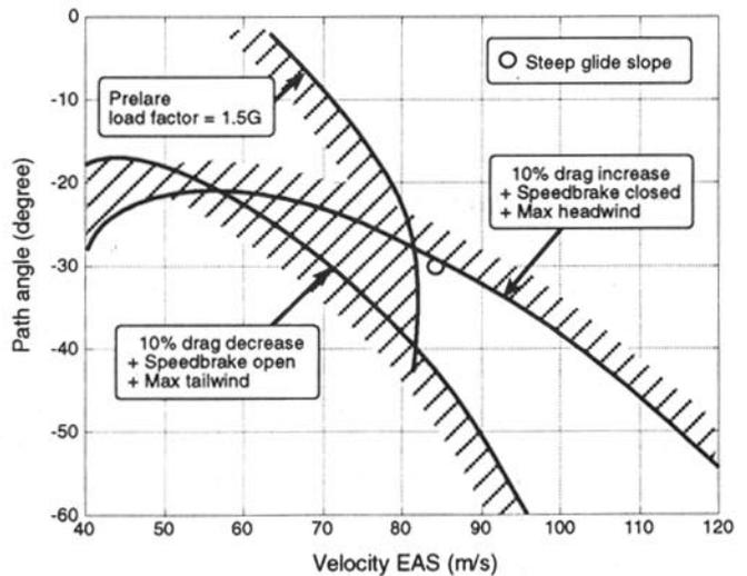
Fig. 5 Velocity vs. flight path angle under the maximum wind conditions. (mass=796kg)
