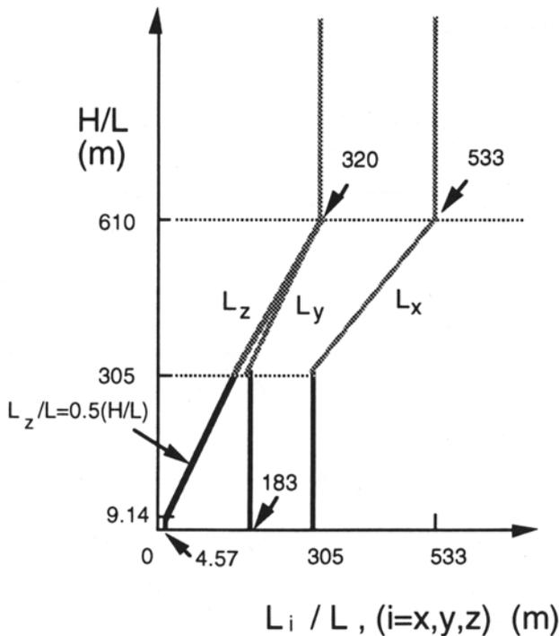
Fig. 4 Scale length of turbulence.  $L_i$
