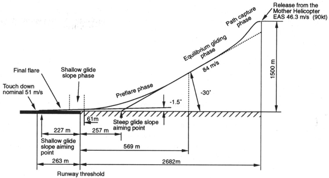
Fig. 6 Reference trajectory.
