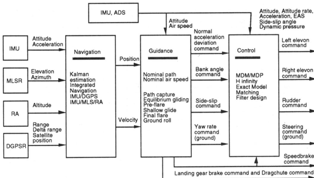
Fig. 7 Function block diagram of GNC system.
