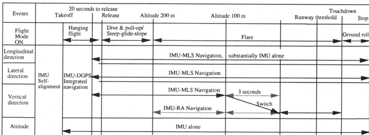
Fig. 9 Integrated navigation switching sequence.
