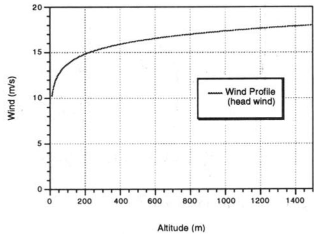
Fig. 1 Maximum steady wind vs altitude.
