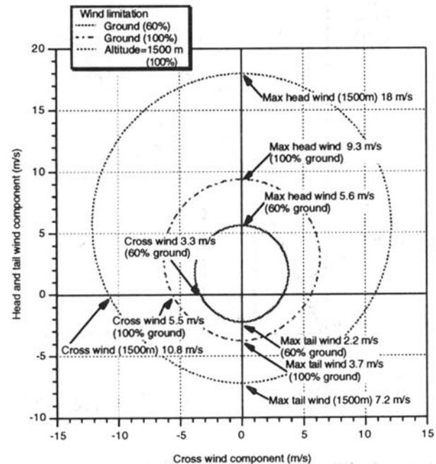
Fig.2 Maximum design wind velocity vs direction.
