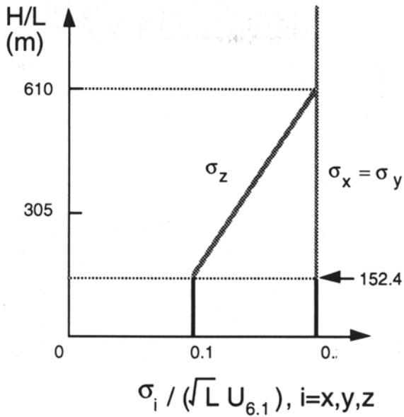
Fig. 3 Intensity of turbulence  $\sigma_i$ .
