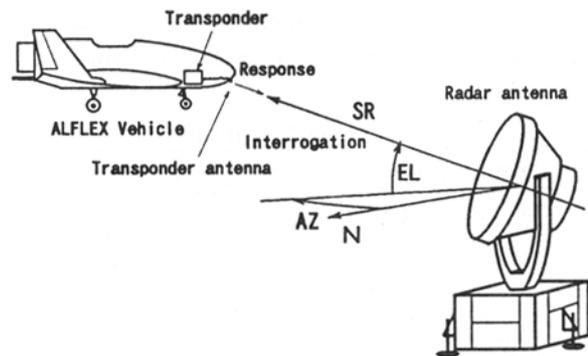
Fig. 2 Positioning using Tracking Radar
