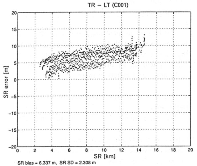
Fig. 4 (c) Calibration Data of SR
