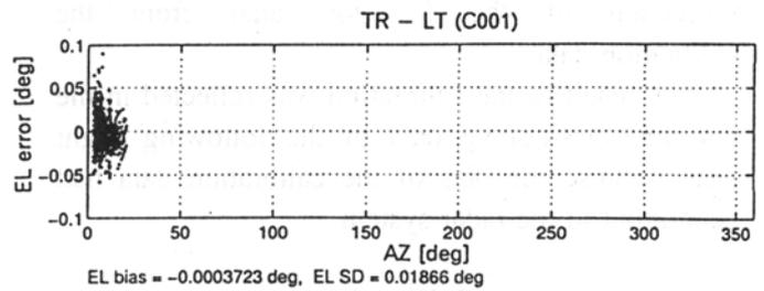
Fig. 4 (b) Calibration Data of EL
