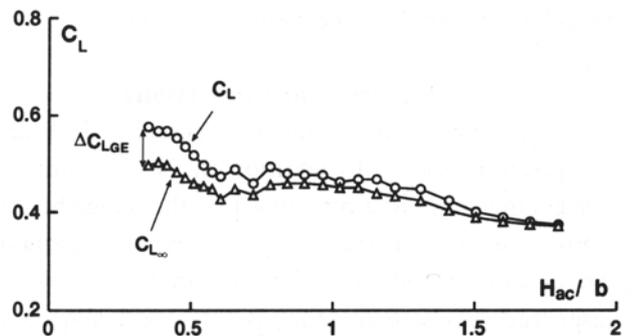
Fig. 4-1 Lift Coefficient during a Landing Approach
