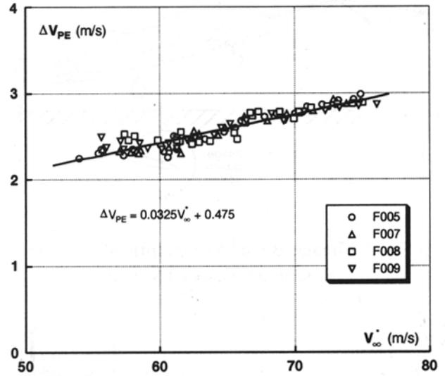
Fig. 3-1 Position Error of Airspeed
