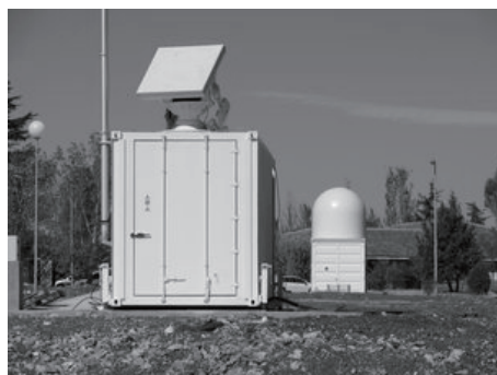
ESA's SSA demonstrator radar
