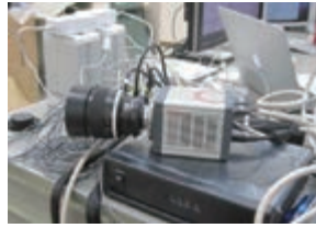
CMOS sensor for detection of LEO objects
