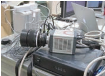
CMOS sensor for LEO observation. Readout time is 60 times faster than that of CCD
