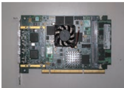
FPGA board H101-PCIXM manufactured by Nallatech.
