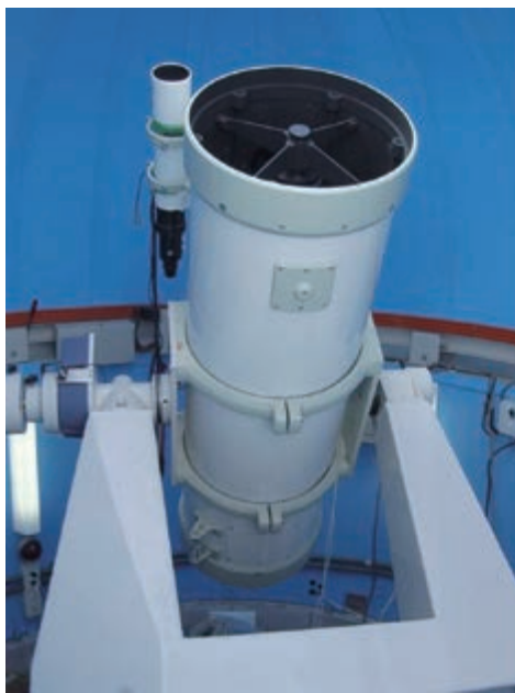
Telescope: Takahashi \epsilon -350 D: 355mm f:1248mm (F/3.6) Equatorial mount: Showa fork-type 25EF
