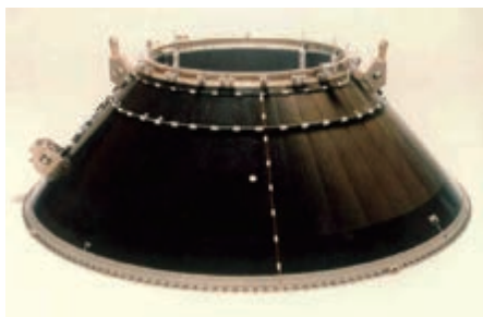
Ariane rocket PAF1194V5 (Ref. Ariane-5 User's Manual Issue 4 Revision 0)
