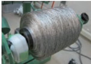
Tether spool ( 2 km Al-SUS tether)
