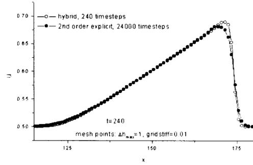
Figure 10: Comparison between the Hybrid and the Explicit schemes for a triangular initial data.
