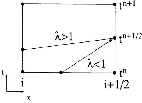
Figure 1: Interpolation scheme of CCG.
