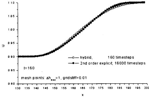
Figure 9: Comparison between the Hybrid and the Explicit Schemes for a forward step-like.
