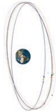
3-D representation of geosynchronous objects detected by the DBAR method from two nights of observations (Aug 18-20, 2012) taken at the Zimmerwald Observatory. (white dot). Both previously cataloged (dotted line) and uncataloged (bold line) objects are shown.
