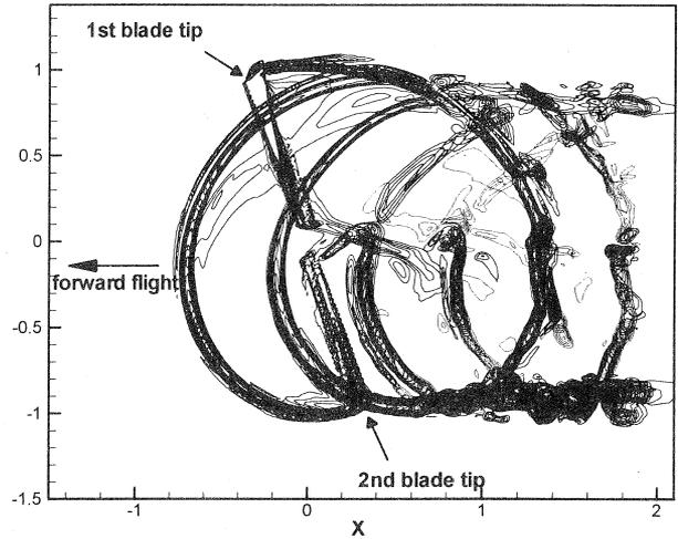
Figure 11. Visualized tip vortices of vorticity contours ( $M=0.8$ ,  $M_{jet}=0.6$ , Normal Jet)
