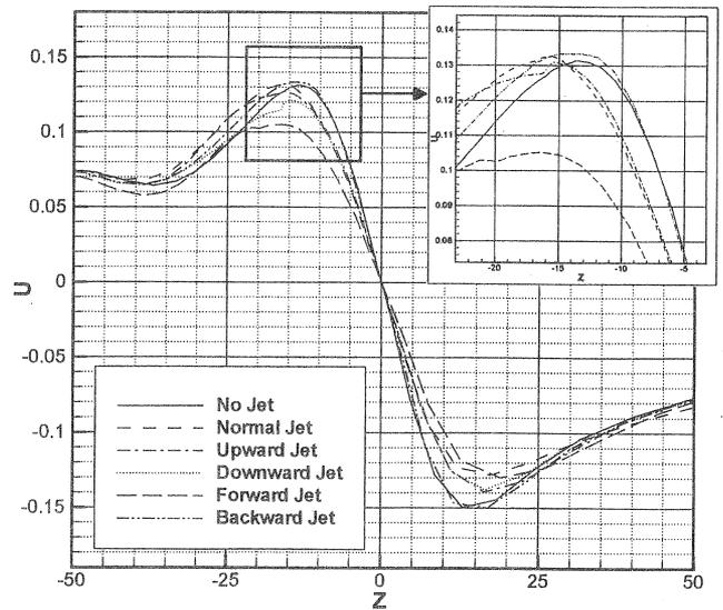
Figure 6. Comparison of tangential velocity distributions at  $L=10C$  according to jet directions ( $M=0.8, M_{jet}=0.6$ )
