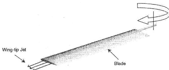
Figure 3. Diagram of wing-tip blowing jet of rotor
