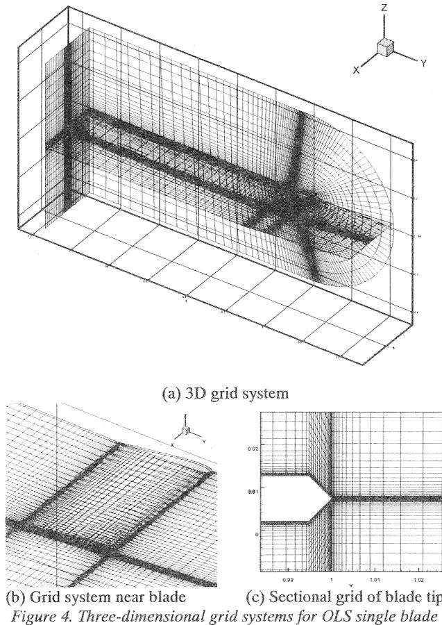
Figure 4. Three-dimensional grid systems for OLS single blade
