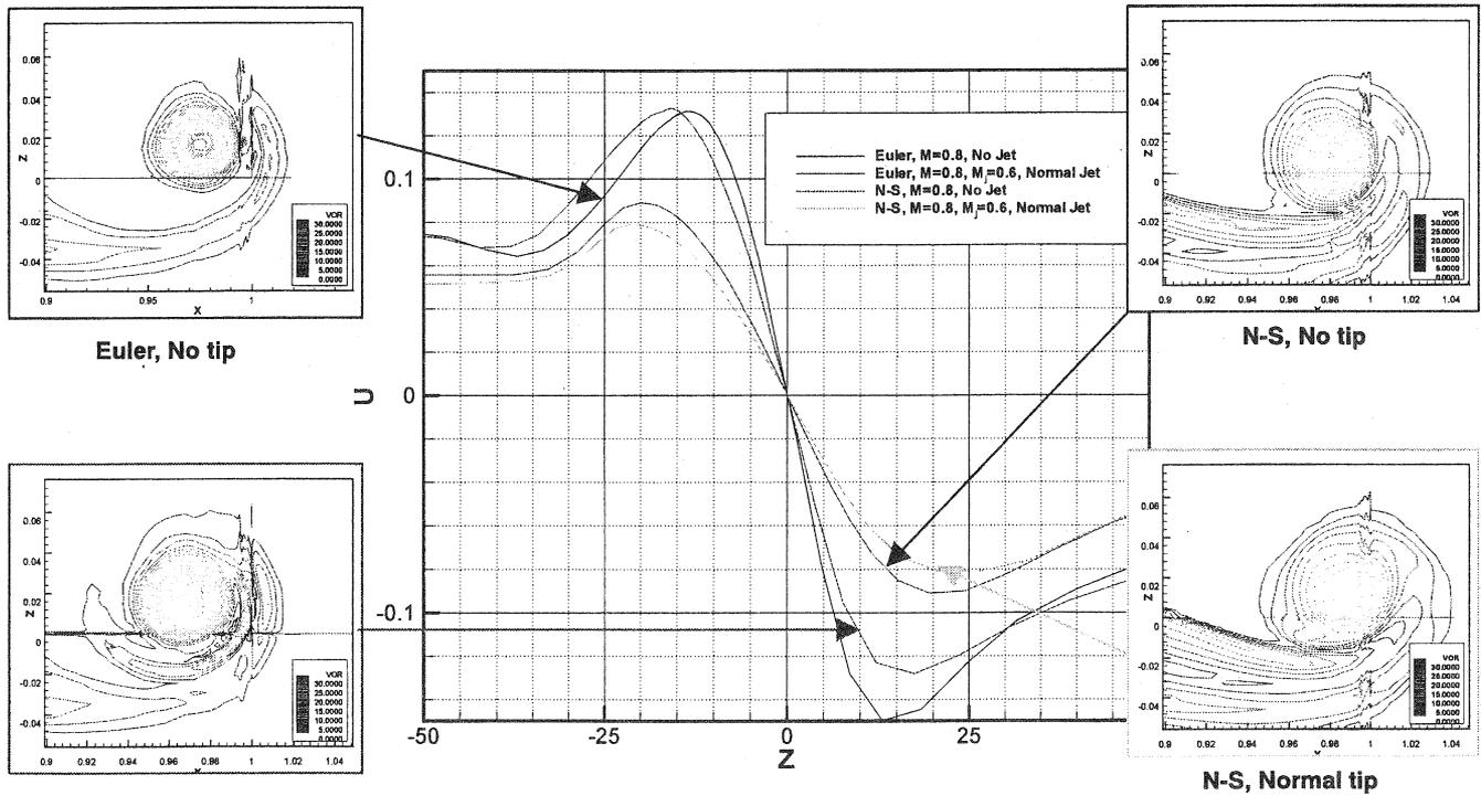
Figure 9. Comparison tangential velocity distributions at  $L=10C$  for inviscid/viscous solutions ( $M=0.8, M_{jet}=0.6$ )
