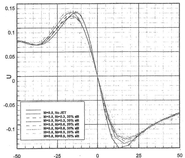
Figure 7. Comparison tangential velocity distributions at  $L=10C$  according to jet Mach number and slit area ( $M=0.8$ )
