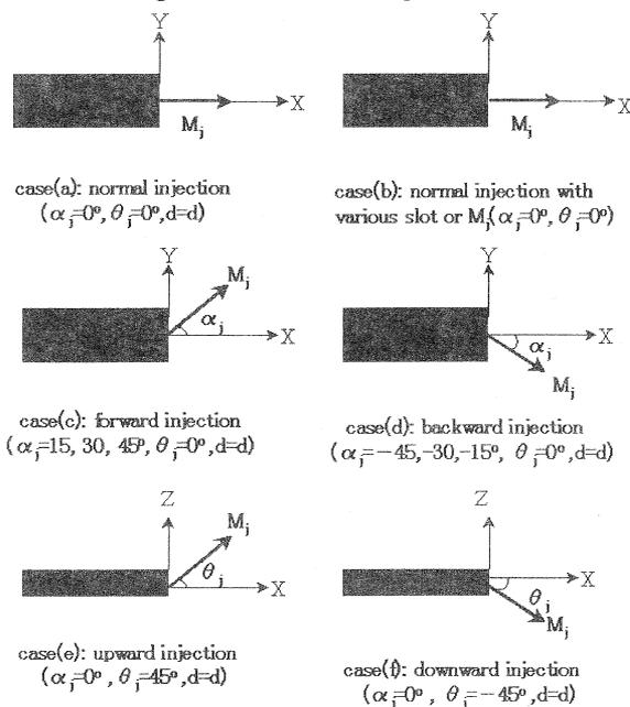
Figure 5. Diagram of cases with various direction of tip jet
