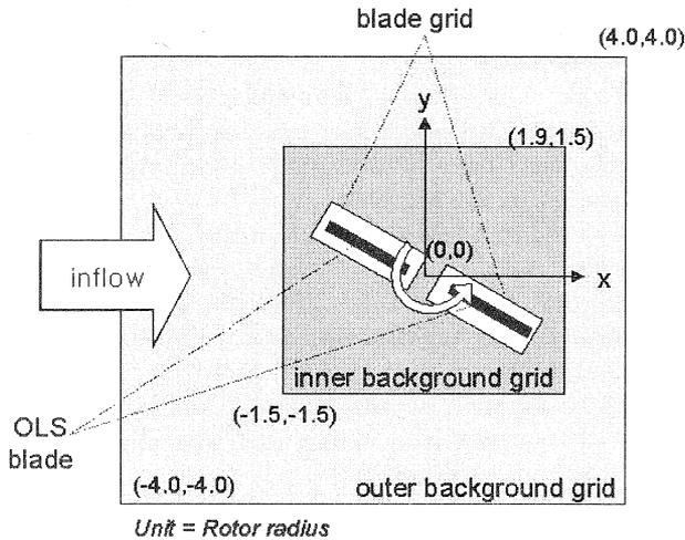
Figure 10. Geometric dimensions of computational domain of inner and outer background grid
