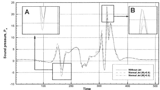
Figure 12. Comparison of sound pressure level (SPL) between cases with overlapped grid system.
