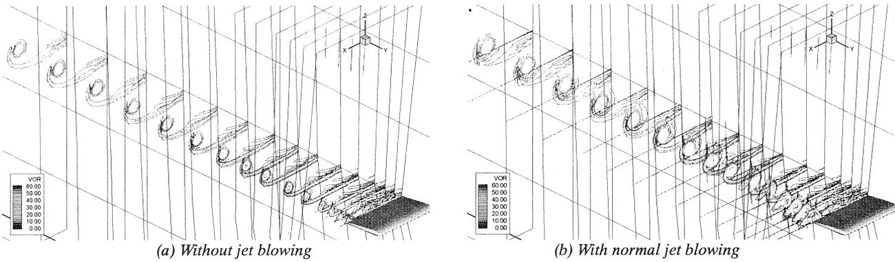
Figure 8. Comparison of vorticity contours up to  $L=10C$  distance for with/without jet blowing ( $M=0.8, M_{jet}=0.6$ )
