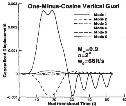
**Fig. 4 Time histories of the structural deformation of the first six modes at  $M_\infty = 0.9$ ,  $\alpha = 2^\circ$**
