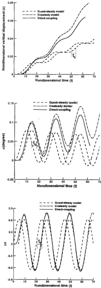
**Fig. 2 Time histories of vertical displacement, angle of attack and incremental load factor for SST at  $M_\infty = 0.9$ ,  $\alpha = 2^\circ$**
