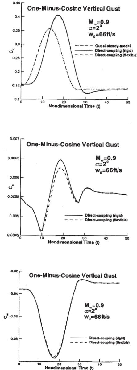
**Fig. 3 Time histories of the coefficients of normal, axial forces and pitching moments for rigid and flexible configurations at  $M_\infty = 0.9$ ,  $\alpha = 2^\circ$**
