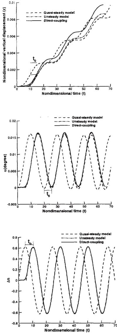
Fig. 1 Time histories of vertical displacement, angle of attack and incremental load factor for SST at  $M_{\infty} = 2.0$ ,  $\alpha = 2^{\circ}$
