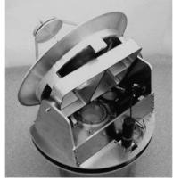
Fig. 3 On board antenna(40cm diameter Ku- Ka band)
