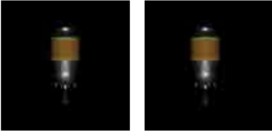
Synthesized stereo images from 50 [meters] distance with FOV 20 [°] lens, base line distance 0.5 [meters] Each projection size of the target: 233x591 [pixels]
