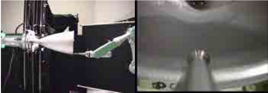
Nozzle probe insert experiment (for DRTS's nozzle) (Corroborate with Tohoku University)
