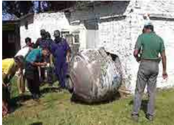
Titanium casing of the STAR-48B solid rocket motor found in northeastern Argentina.
