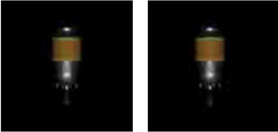
Synthesized stereo images from 50 [meters] distance with FOV 20 [°] lens, base line distance 0.5 [meters]
