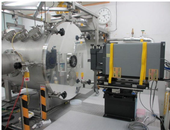
a. Space chamber and laser interferometer
