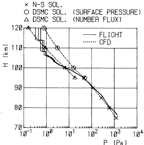
Fig. 30 High-altitude pressure for altitude
