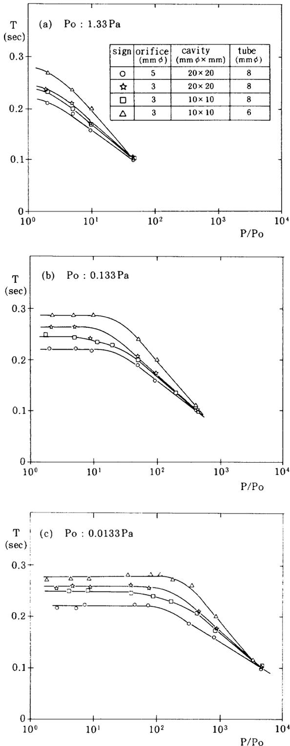
Fig. 10 Set pressure (90%) and response time
