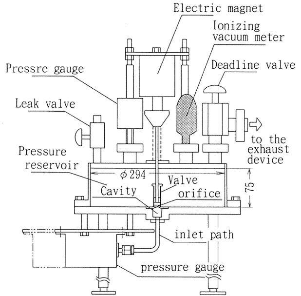
Fig. 8 Details of pressure-response test unit
