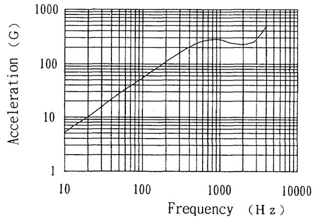
Fig. 20 Acceleration in an impact test (Y axis "+") with frequency
