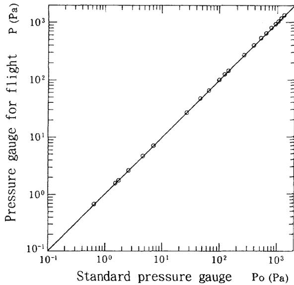
Fig. 22 Calibration result of pressure gauge for flight
