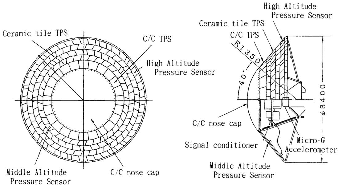
Fig. 2 Schematic diagram of OREX vehicle
