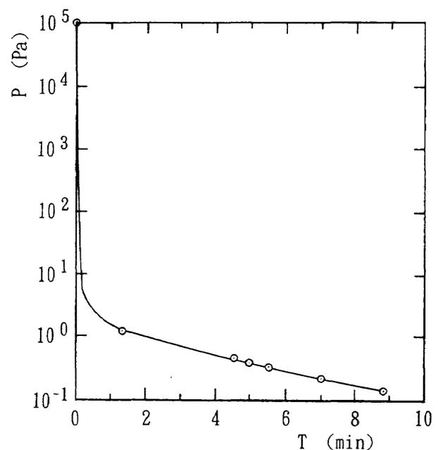
Fig. 24 Diagram of exhaust characteristics of pressure confirmation test unit
