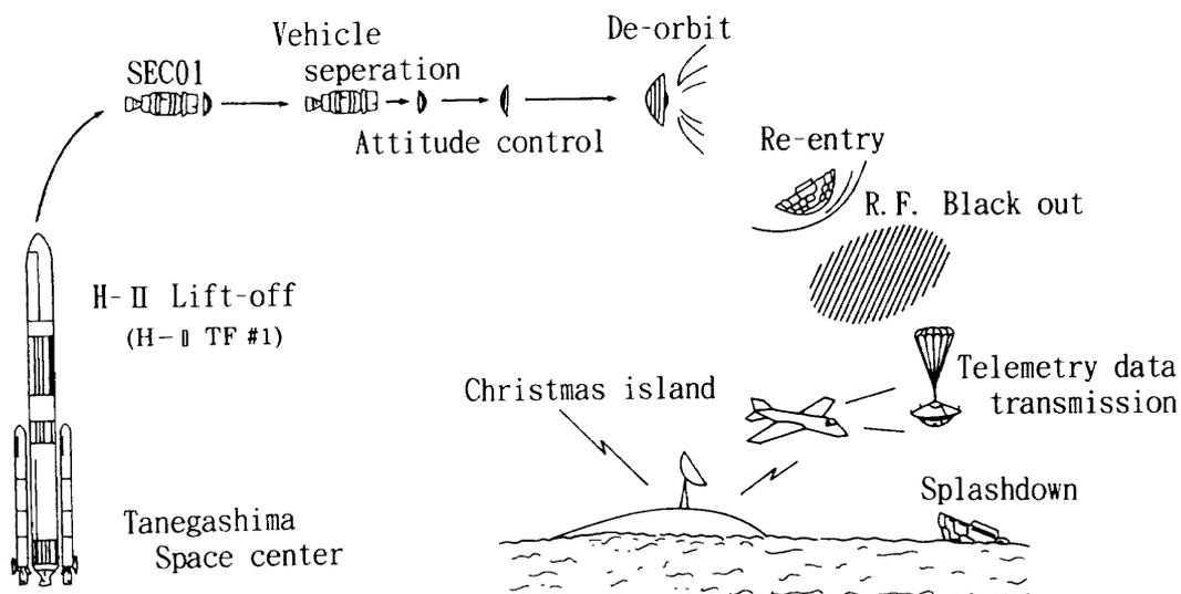
Fig. 1 Sketch of OREX flight profile
