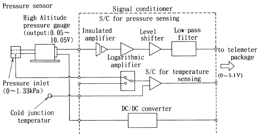
Fig. 14 Functional block diagram of signal conditioner
