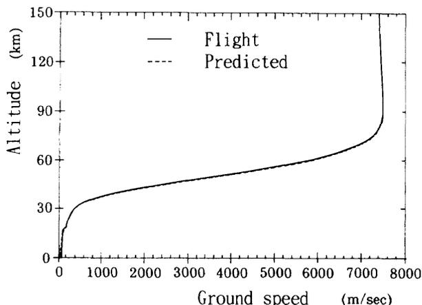
Fig. 28 Ground speed versus altitude
