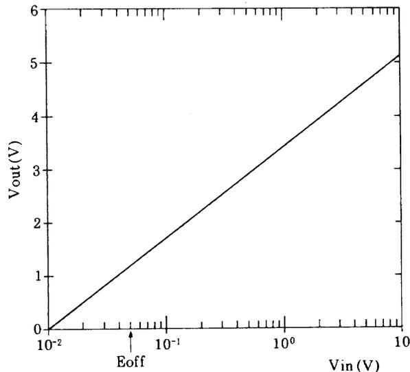
Fig. 13 Characteristics of signal conditioner
