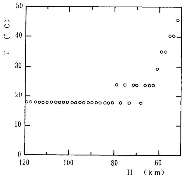
Fig. 27 Temperature of pressure inlet with altitude
