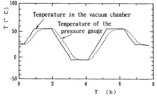
Fig. 17 Pressure gauge temperature cycle test
