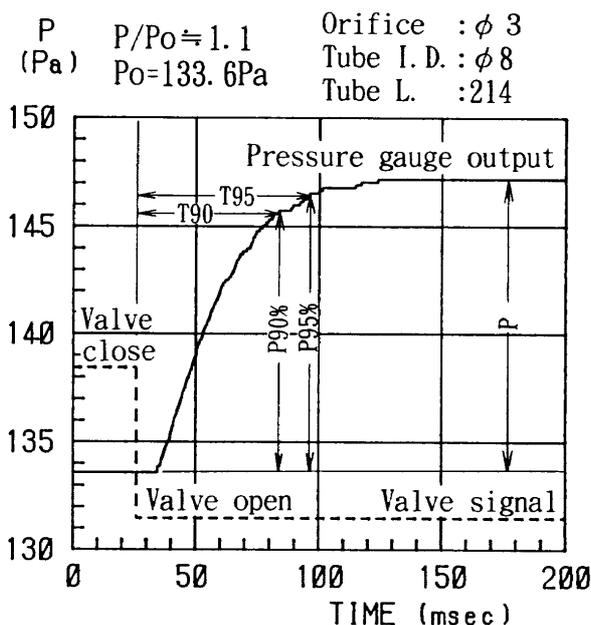
Fig. 11 Time-dependent change of pressure gauge output for step input
