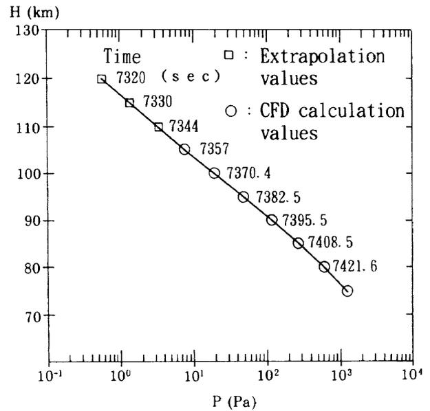
Fig. 3 High-altitude wall surface pressure versus altitude
