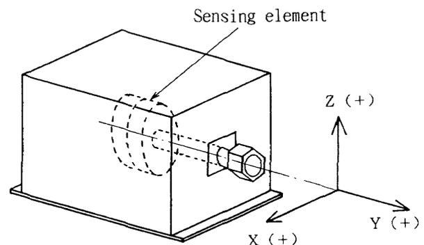
Fig. 15 Definition of triaxial direction in vibration/shock test
