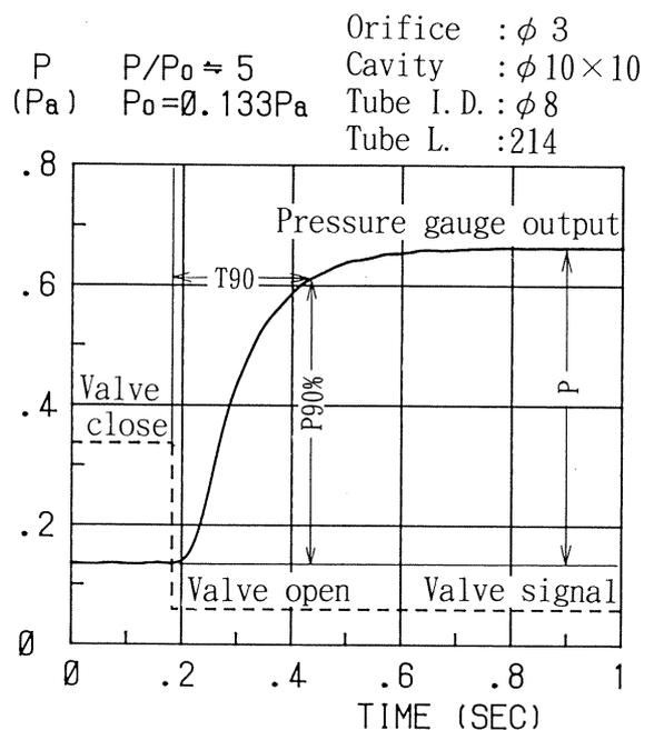
Fig. 9 Time-dependent change of pressure gauge output
