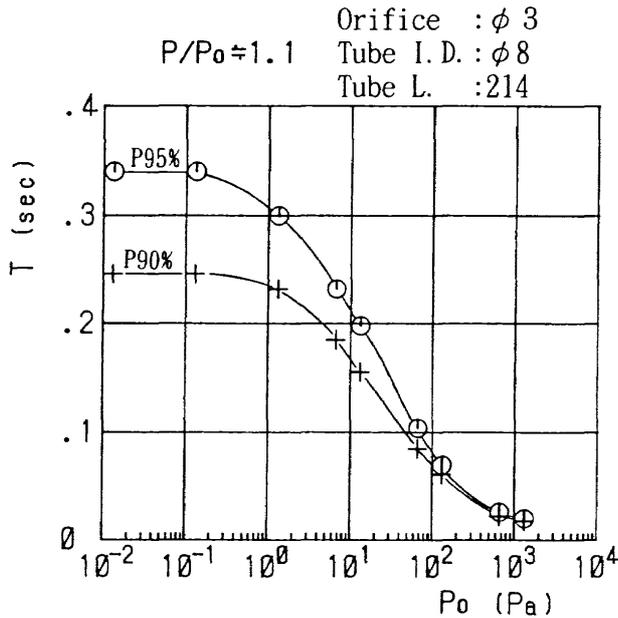
Fig. 12 High-altitude wall surface pressure and response time
