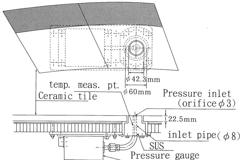
Fig. 6 Outline of pressure sensor system
