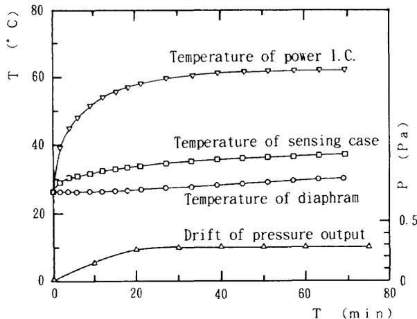
Fig. 16 Pressure sensor temperature distribution characteristics/drift characteristics
