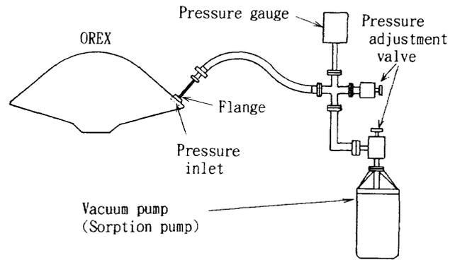
Fig. 23 Schematic diagram of pressure confirmation test unit
