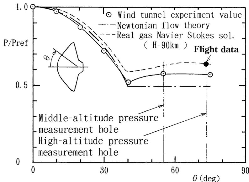
Fig. 32 OREX wall surface pressure distribution
