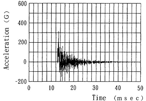
Fig. 19 Acceleration in an impact test (Y axis "+") with time
