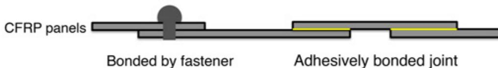
Researches for realizing more effective joints and adhesions are being done.
