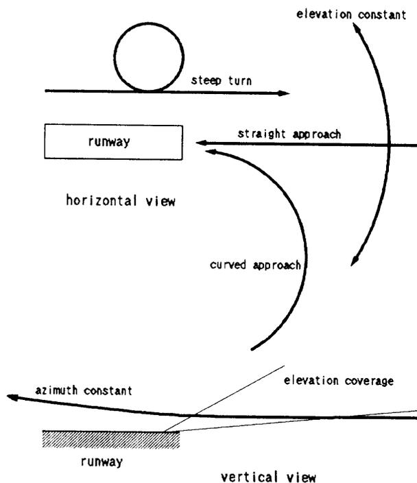
Figure 3.3 flight test pattern
