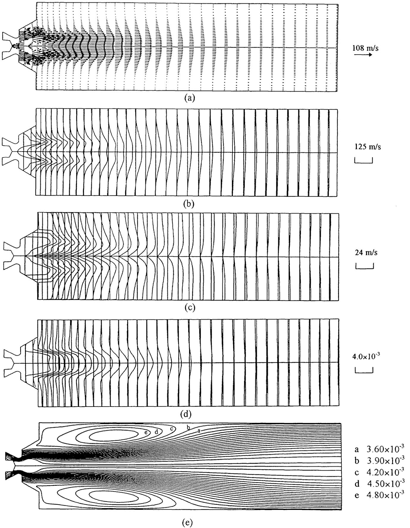
Fig. 23 Predicted results with the standard  $\kappa$ - $\epsilon$  model for Case 6 (a) velocity vectors, (b) axial velocity, (c) tangential velocity, (d) fuel concentration, (e) stream functions
