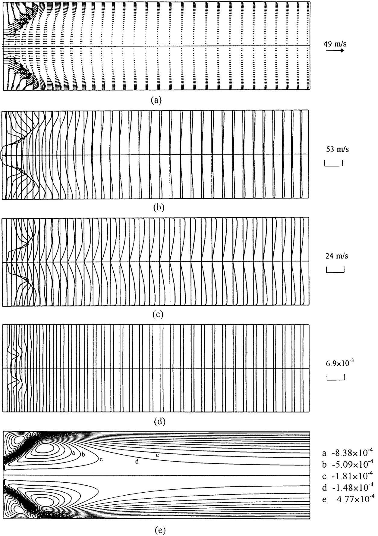
Fig. 15 Predicted results with the standard  $\kappa$ - $\epsilon$  model for Case 10 (a) velocity vectors, (b) axial velocity, (c) tangential velocity, (d) fuel concentration, (e) stream functions
