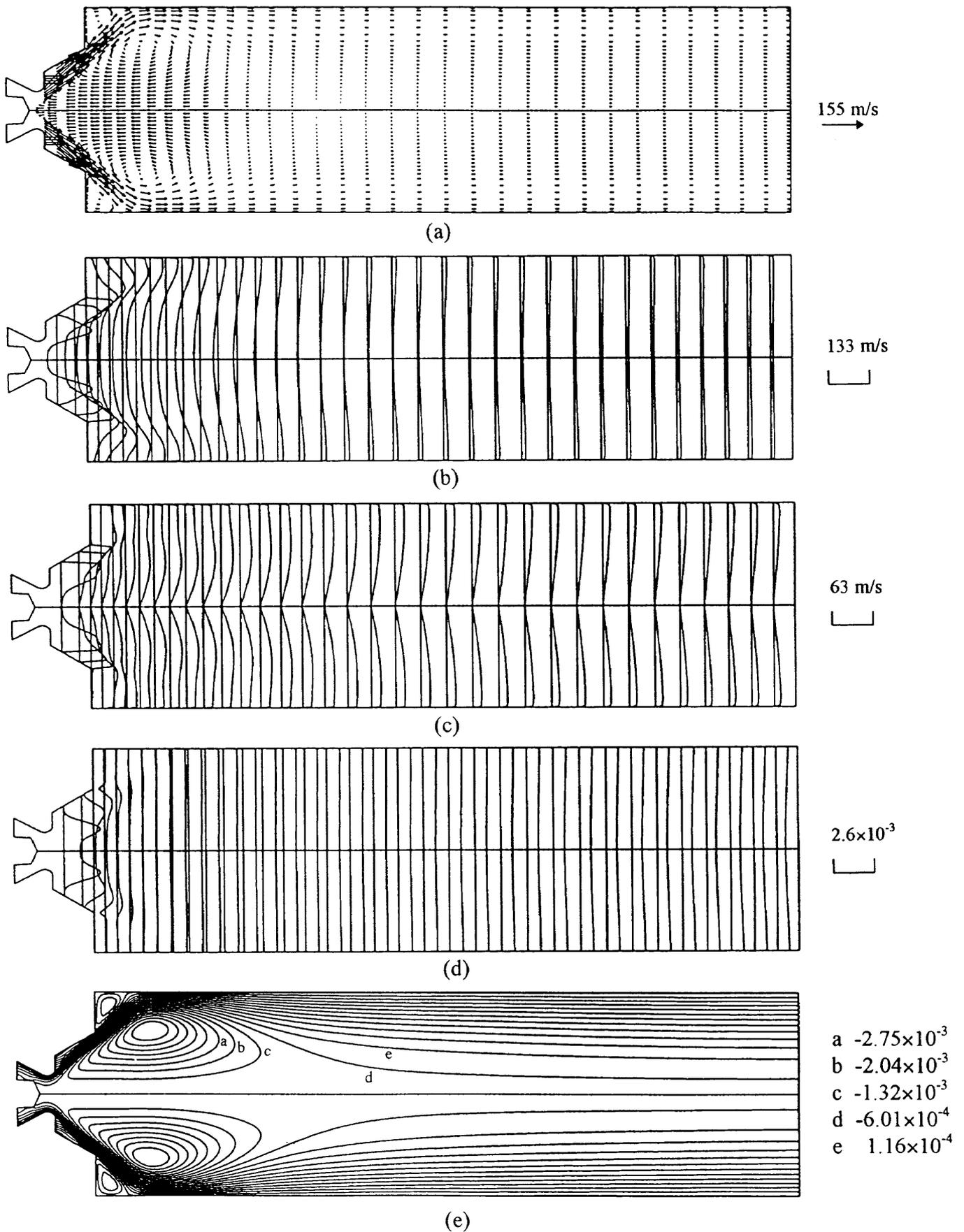
Fig. 24 Predicted results with the standard  $\kappa$ - $\epsilon$  model for Case 7 (a) velocity vectors, (b) axial velocity, (c) tangential velocity, (d) fuel concentration, (e) stream functions
