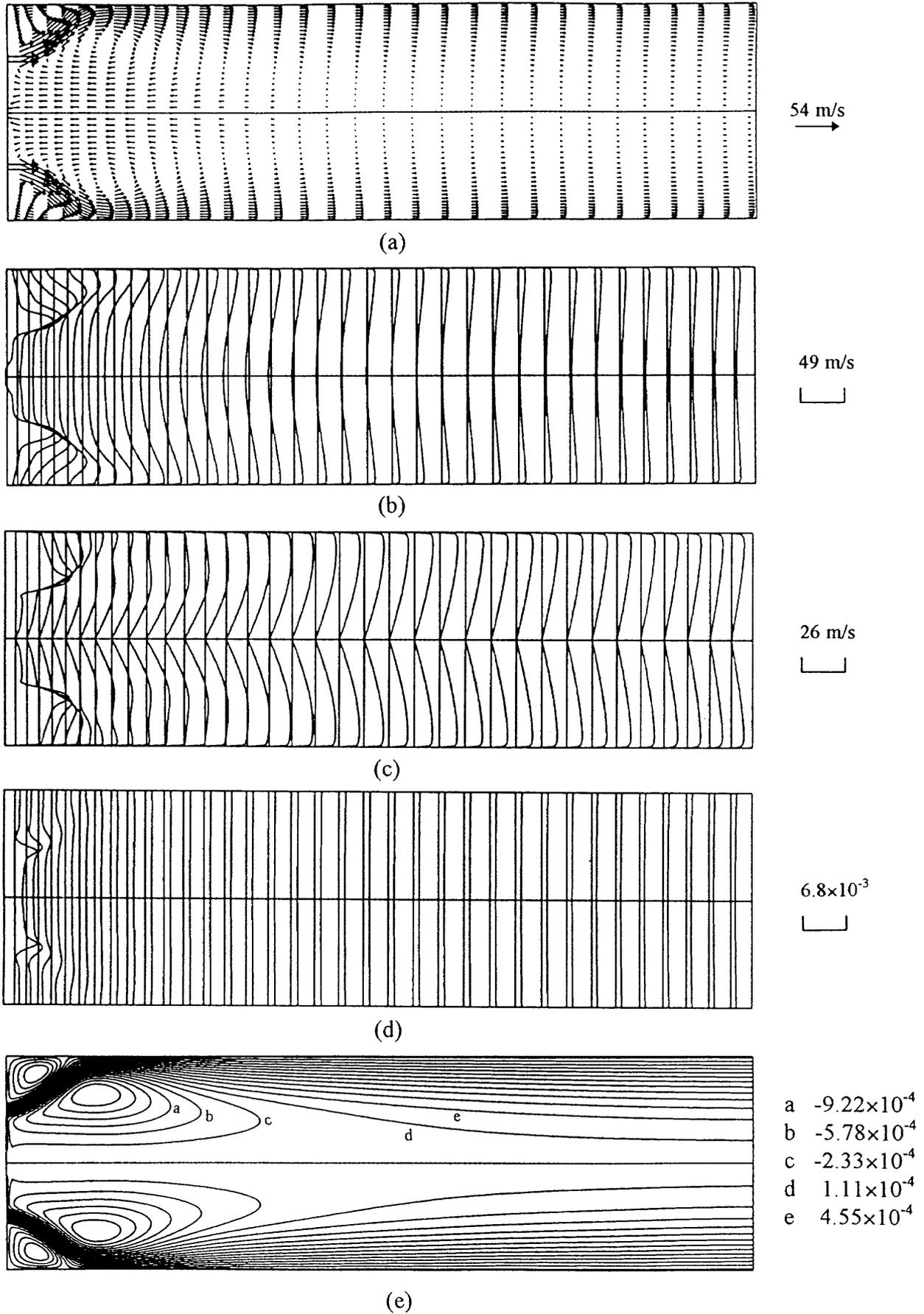
Fig. 13 Predicted results with the standard  $\kappa$ - $\epsilon$  model for Case 8 (a) velocity vectors, (b) axial velocity, (c) tangential velocity, (d) fuel concentration, (e) stream functions
