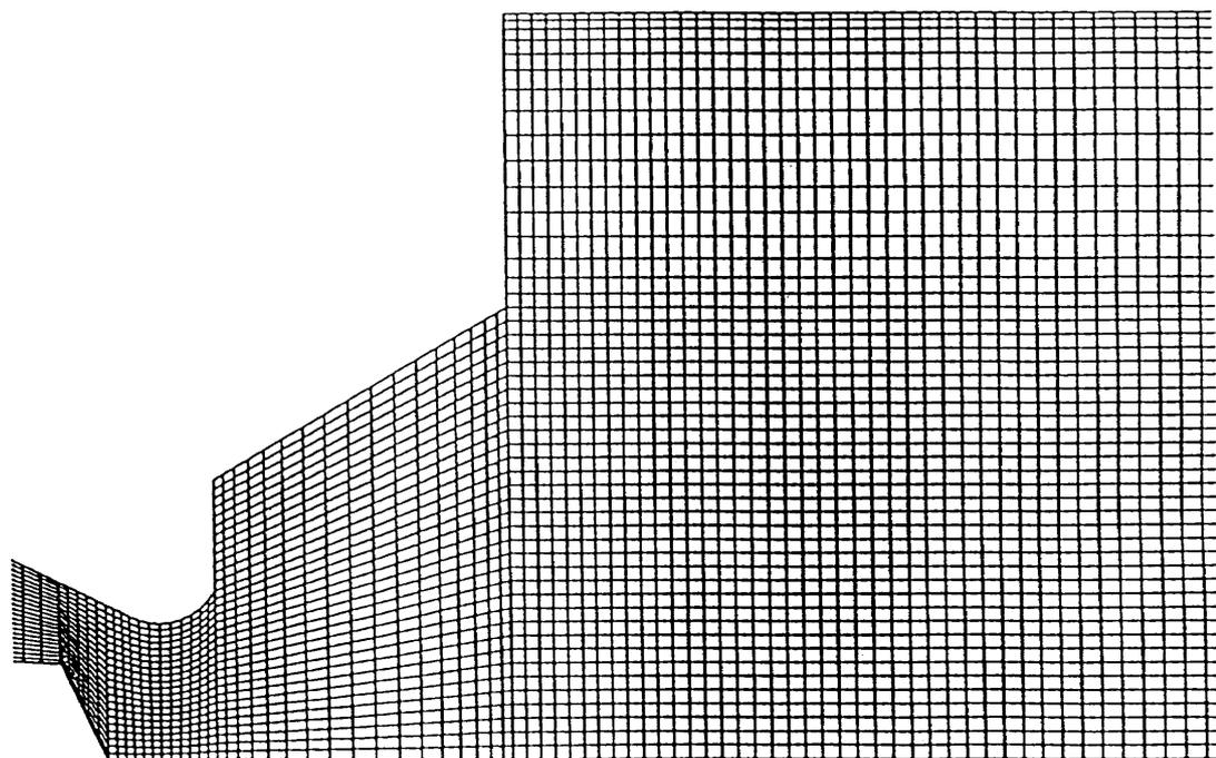
Fig. 5 The grid system in the double swirler
