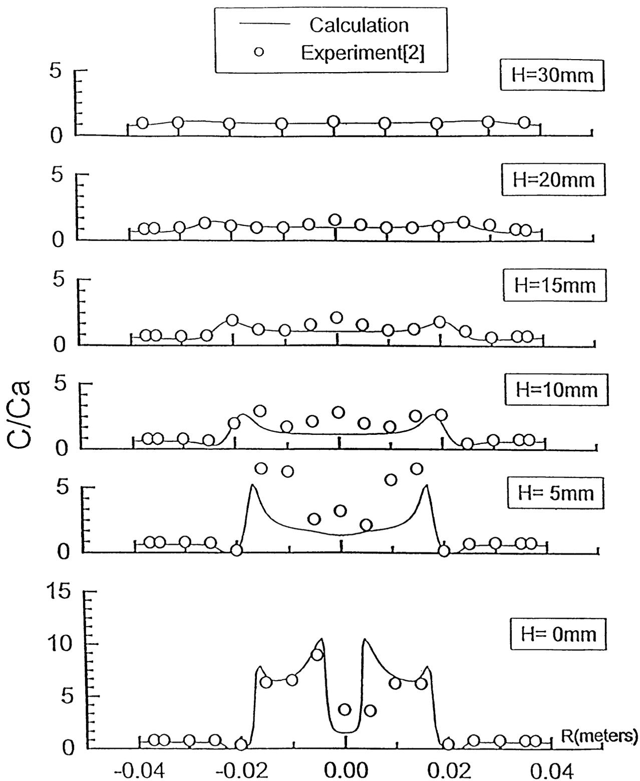
Fig. 14 Comparison of predictions and experiment data for fuel concentration distribution (Case 8)
