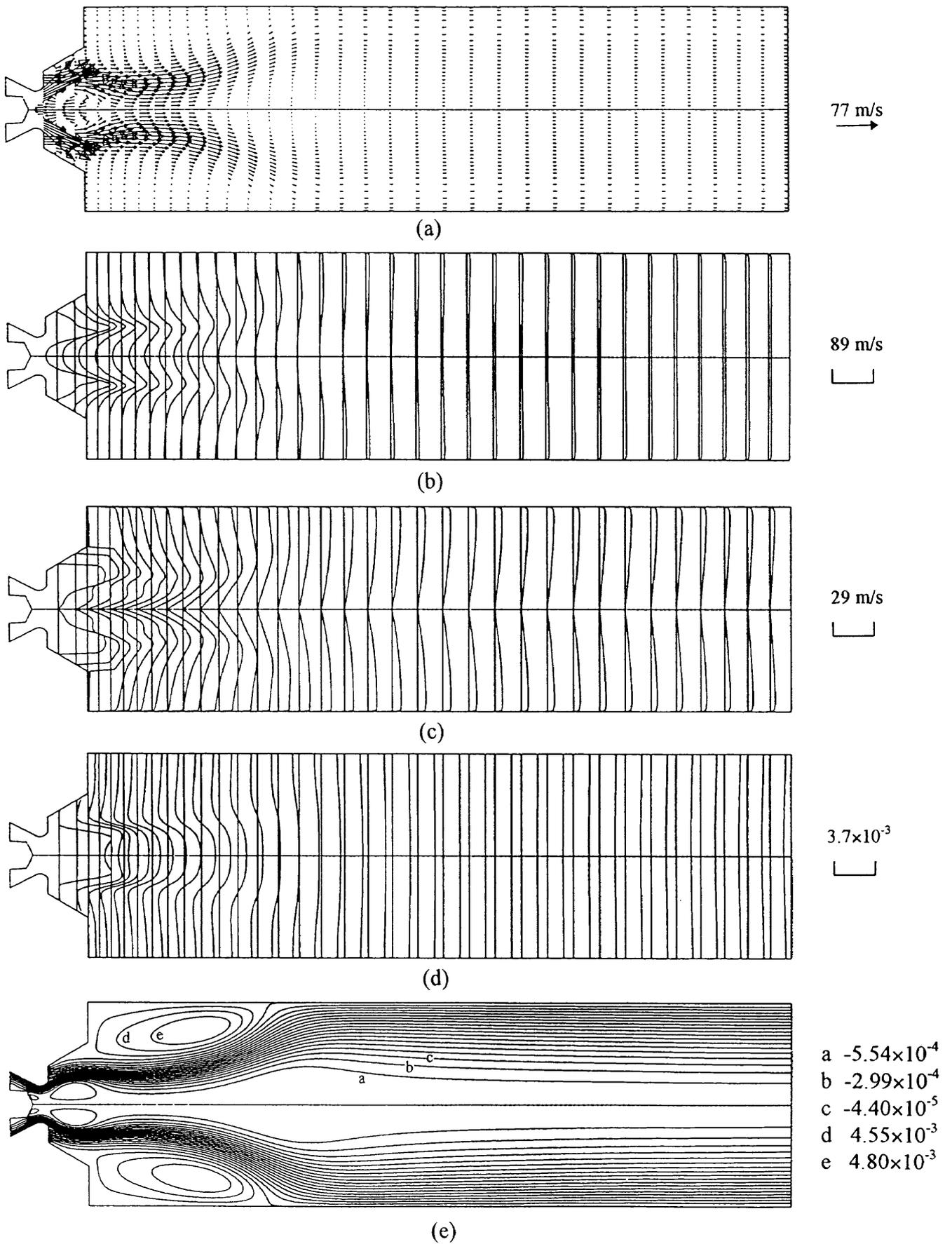
Fig. 22 Predicted results with the standard  $\kappa$ - $\epsilon$  model for Case 5 (a) velocity vectors, (b) axial velocity, (c) tangential velocity, (d) fuel concentration, (e) stream functions
