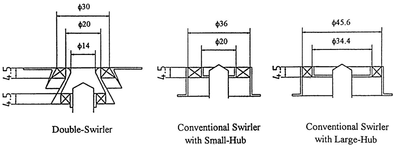
Fig. 2 Differential swirler configurations used in the burner
