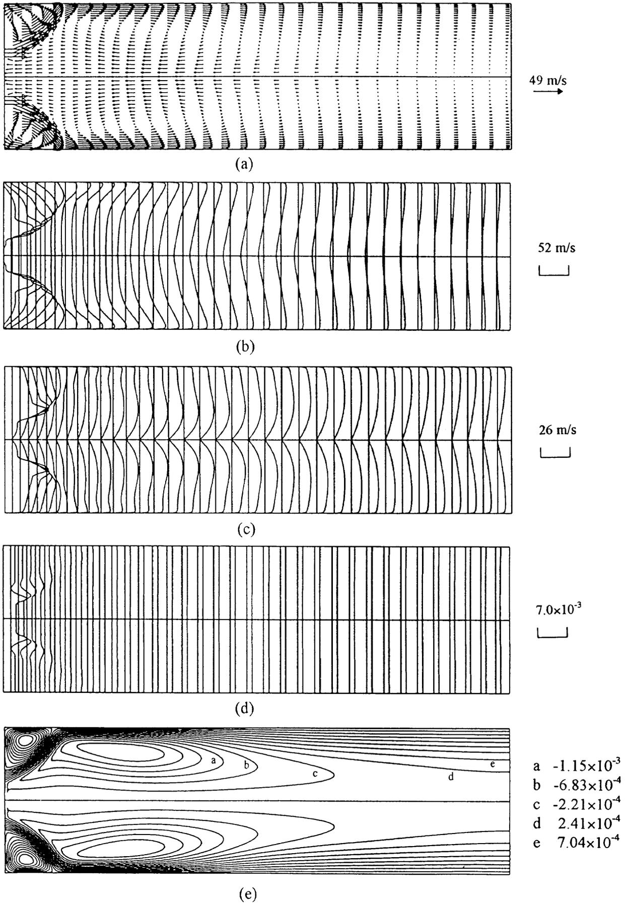
Fig. 16 Predicted results with the RNG  $\kappa$ - $\epsilon$  model for Case 10 (a) velocity vectors, (b) axial velocity, (c) tangential velocity, (d) fuel concentration, (e) stream functions
