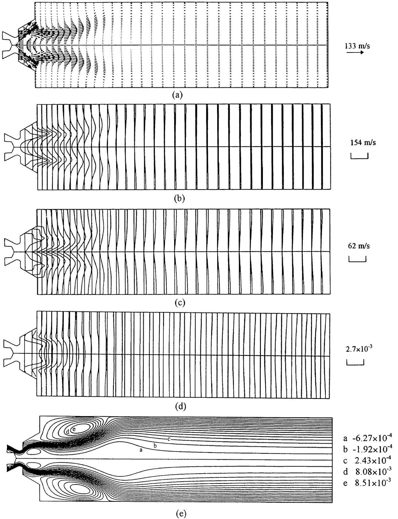
Fig. 20 Predicted results with the standard  $\kappa$ - $\epsilon$  model for Case 3 (a) velocity vectors, (b) axial velocity, (c) tangential velocity, (d) fuel concentration, (e) stream functions
