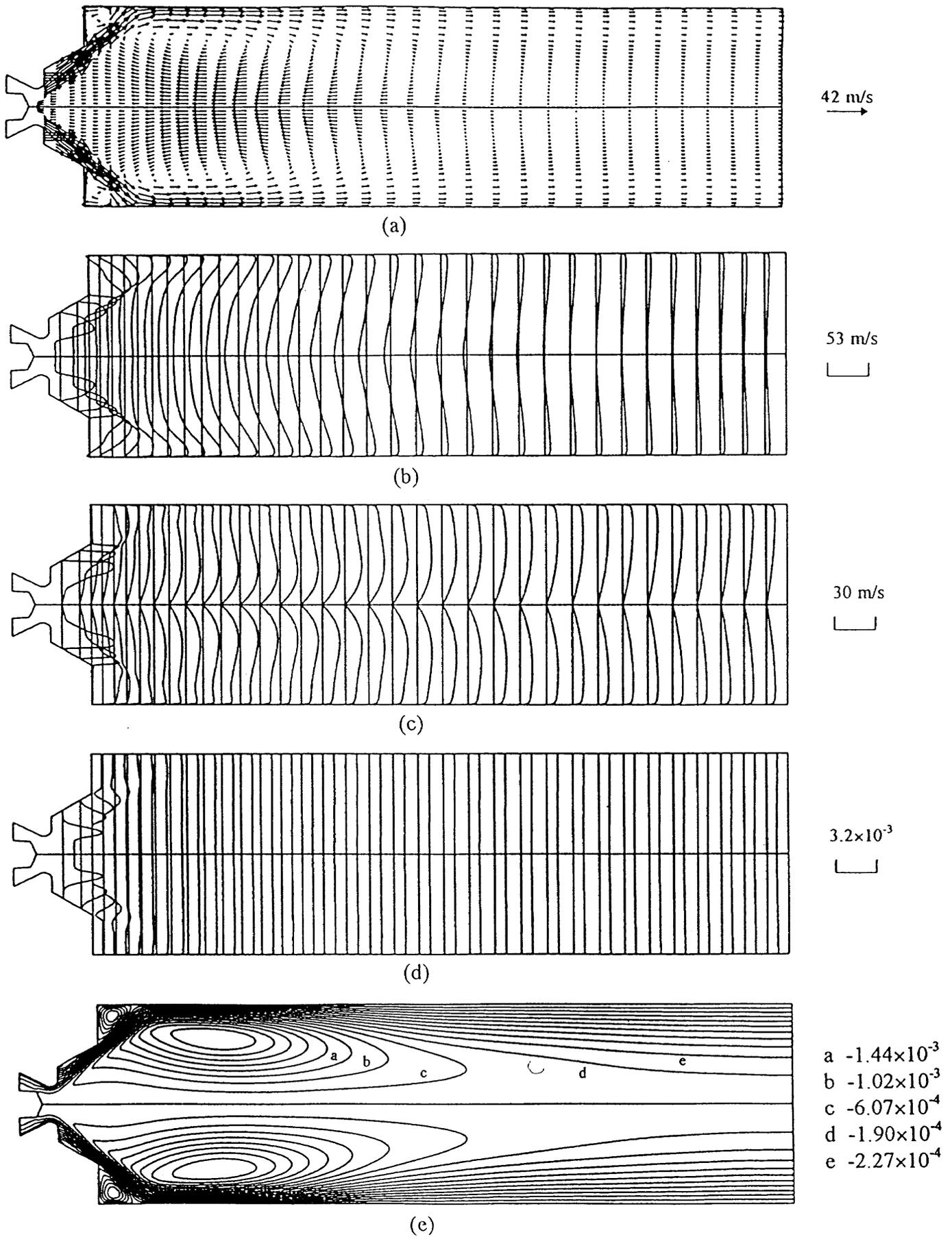
Fig. 8 Predicted results with the RNG  $\kappa$ - $\epsilon$  model for Case 1 (a) velocity vectors, (b) axial velocity, (c) tangential velocity, (d) fuel concentration, (e) stream functions
