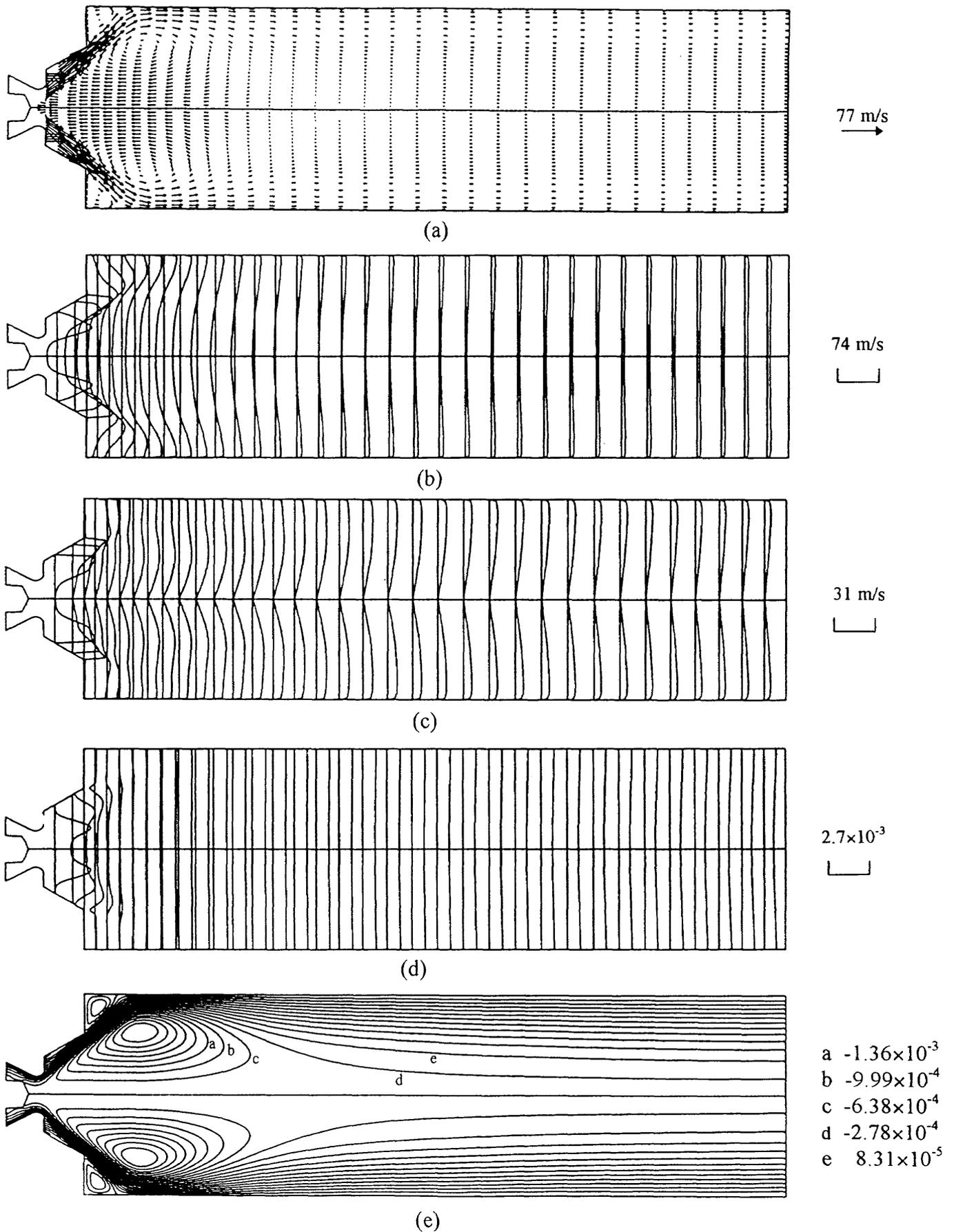
Fig. 21 Predicted results with the standard  $\kappa$ - $\epsilon$  model for Case 4 (a) velocity vectors, (b) axial velocity, (c) tangential velocity, (d) fuel concentration, (e) stream functions
