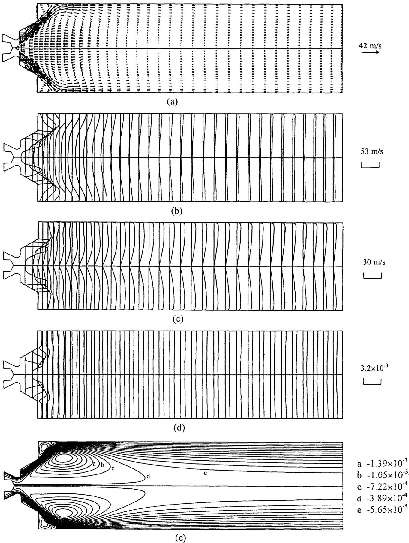
Fig. 6 Predicted results with the standard  $\kappa$ - $\epsilon$  model for Case 1 (a) velocity vectors, (b) axial velocity, (c) tangential velocity, (d) fuel concentration, (e) stream functions
