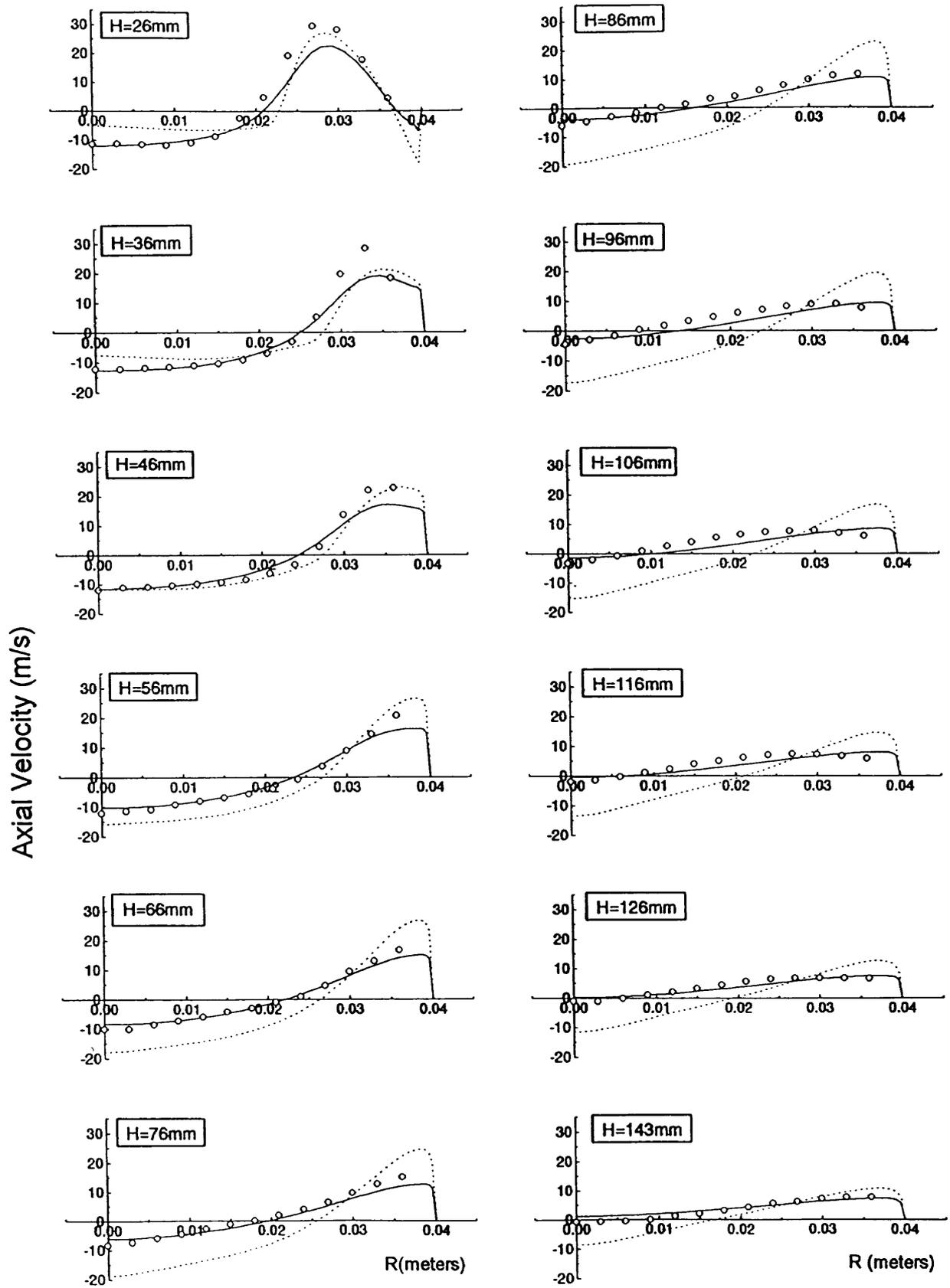
Fig. 9 Comparisons of prediction and experiment data for axial velocity distribution (—  $\kappa\text{-}\epsilon$  model - - - RNG  $\kappa\text{-}\epsilon$  model  $\circ$  experiment)
