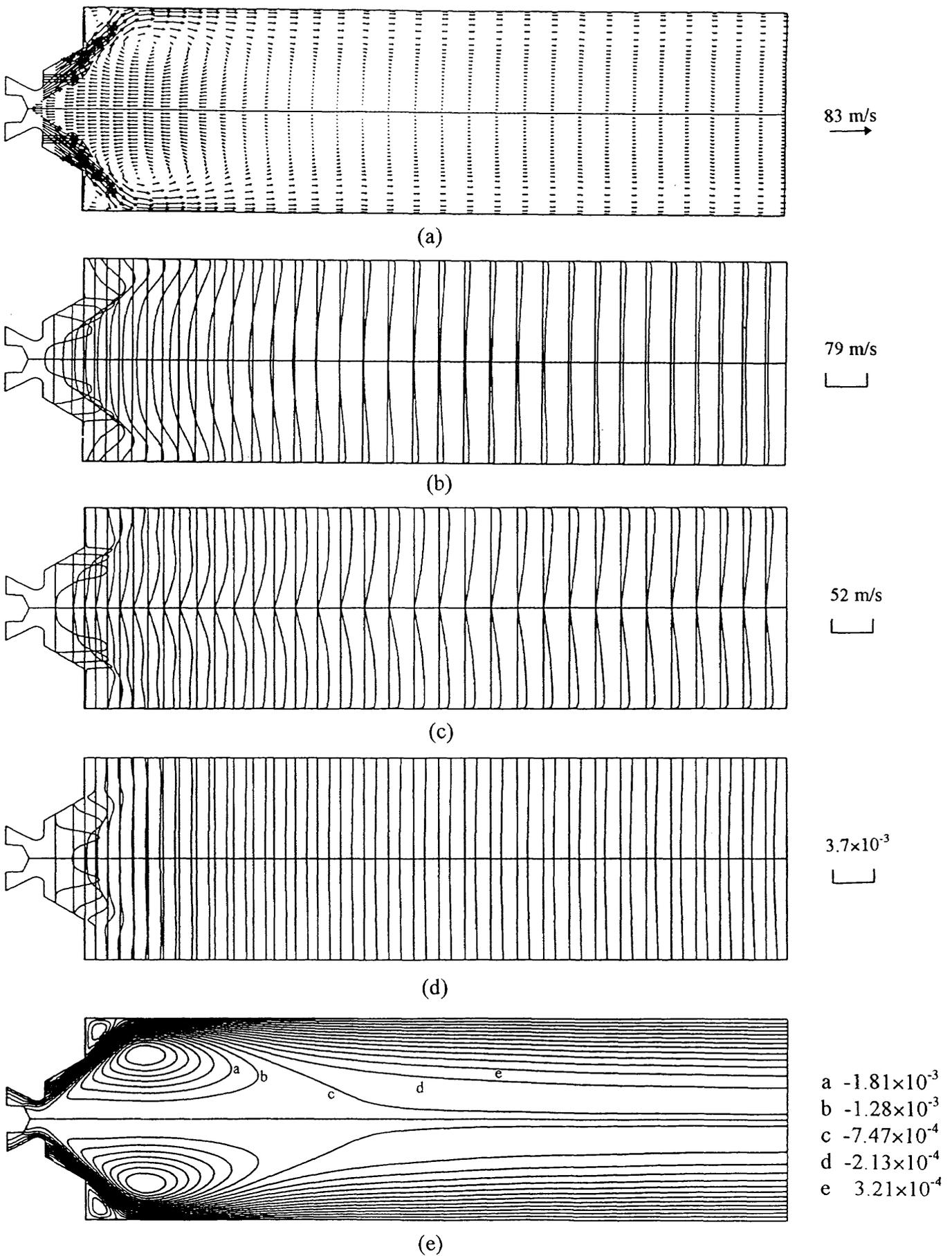
Fig. 19 Predicted results with the standard  $\kappa$ - $\epsilon$  model for Case 2 (a) velocity vectors, (b) axial velocity, (c) tangential velocity, (d) fuel concentration, (e) stream functions
