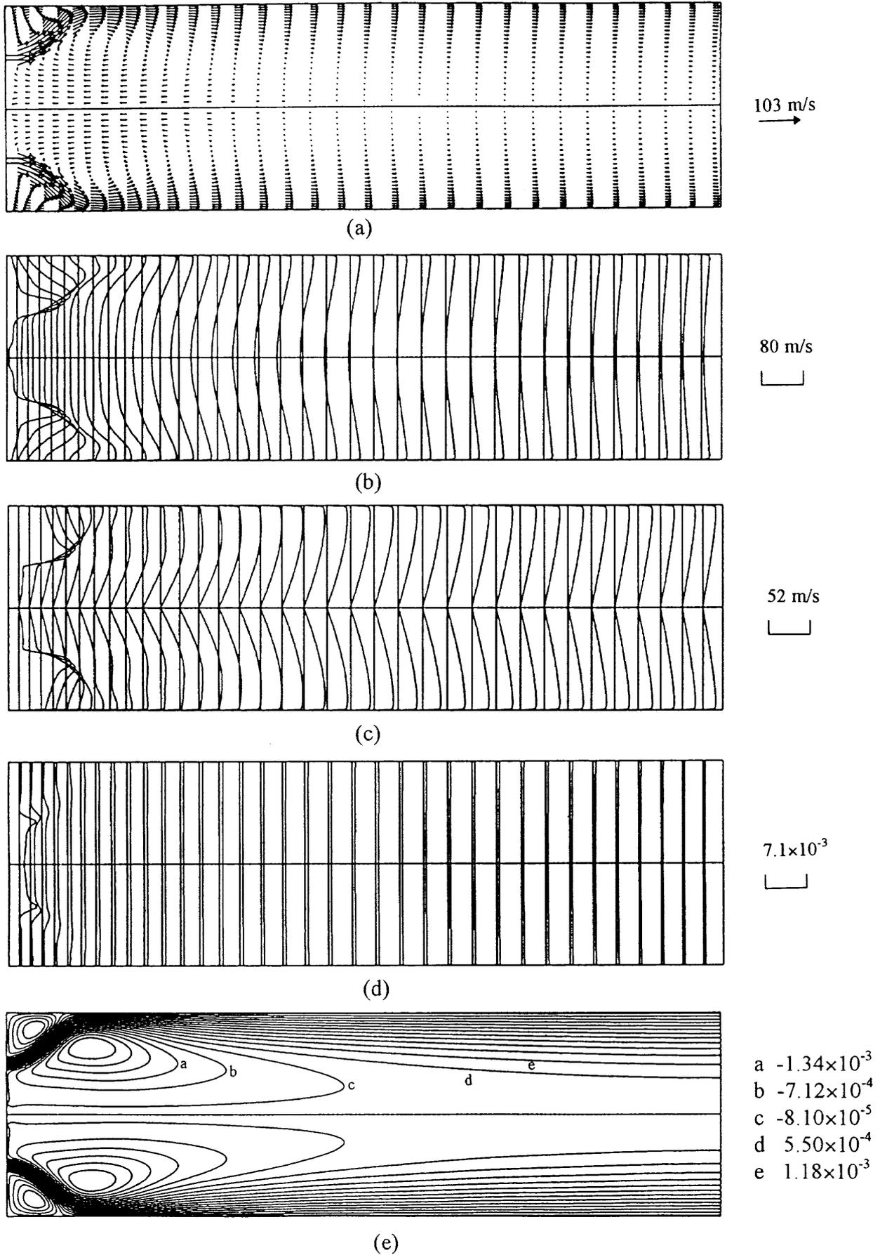
Fig. 25 Predicted results with the standard  $\kappa$ - $\epsilon$  model for Case 9 (a) velocity vectors, (b) axial velocity, (c) tangential velocity, (d) fuel concentration, (e) stream functions
