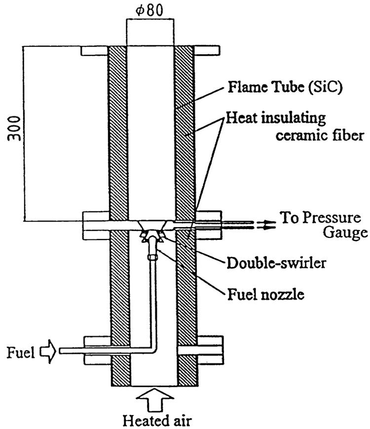
Fig. 1 Schematic diagram of flow system
