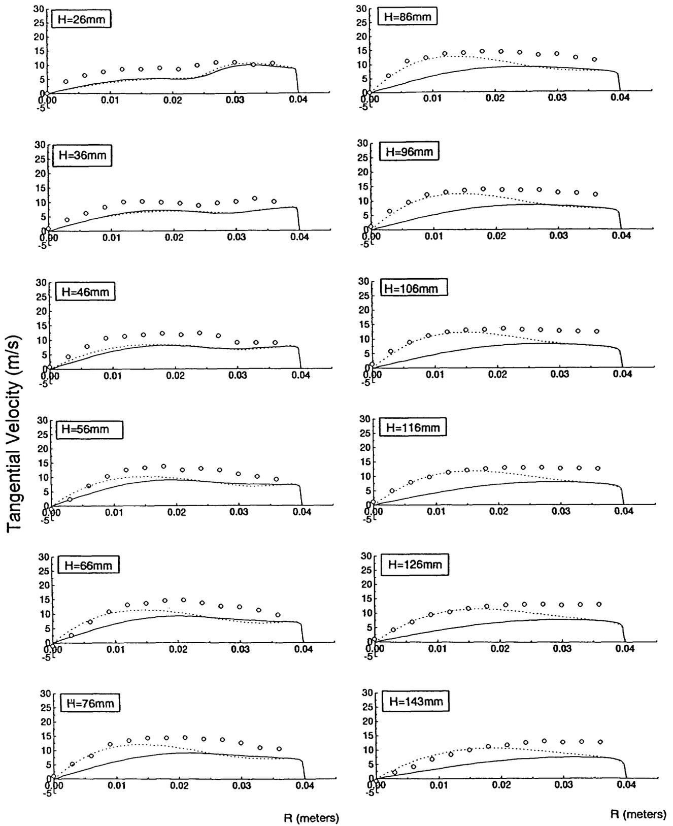
Fig. 10 Comparisons of prediction and experiment data for tangential velocity distribution
