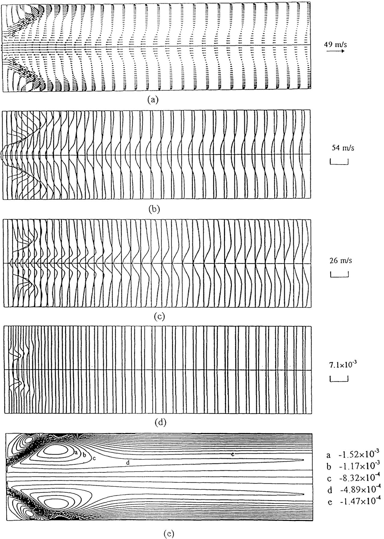
Fig. 17 Predicted results with the RSM for Case 10 (a) velocity vectors, (b) axial velocity, (c) tangential velocity, (d) fuel concentration, (e) stream functions
