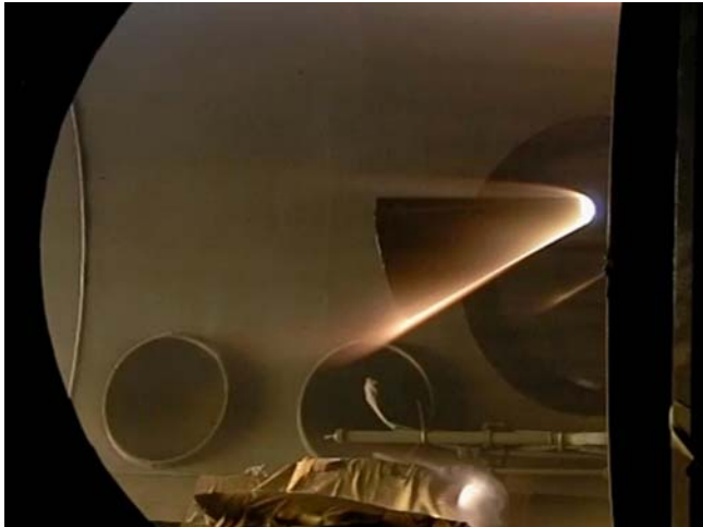
Figure.7 A photograph of the blunted cone just flying in the HUEST test section. Hypersonic test flow ( V_\infty=5\text{km/s} ) came from right to left. Strong luminosity was observed during test.
