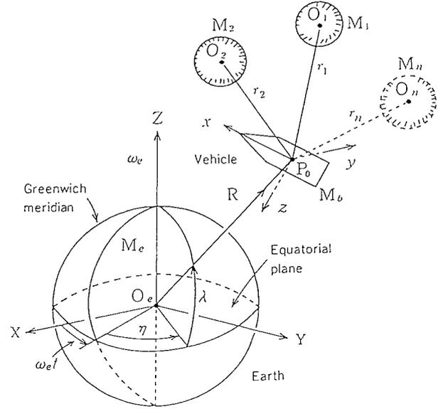
Fig. 1 Inertial Reference Coordinate ( $O_e$ -XYZ) and body-fixed coordinate ( $P_0$ -xyz)
