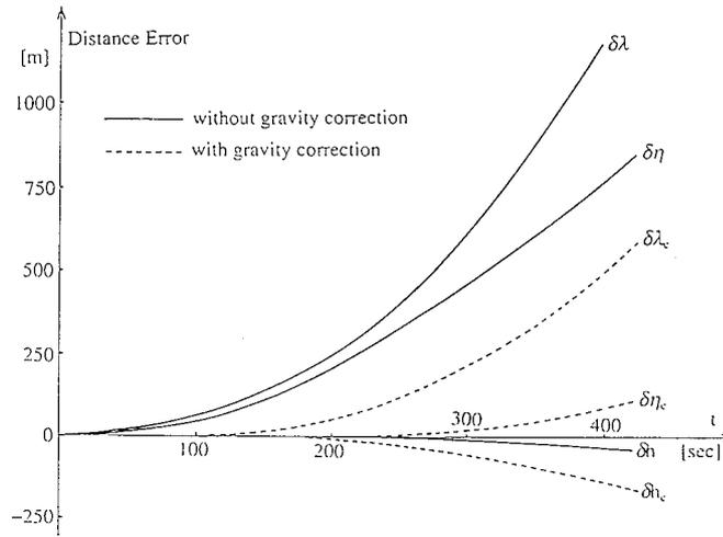
Fig. 7 Navigation errors due to unpredictable body (model-1)
