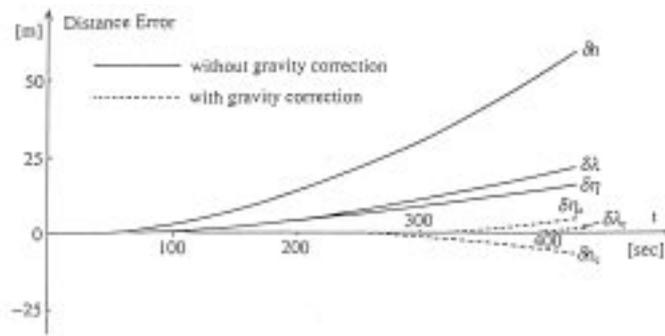
Fig. 8 Navigation errors due to unpredictable body (model-2)
