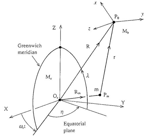
Fig. 6 Position relation among vehicle, earth and unpredictable body
