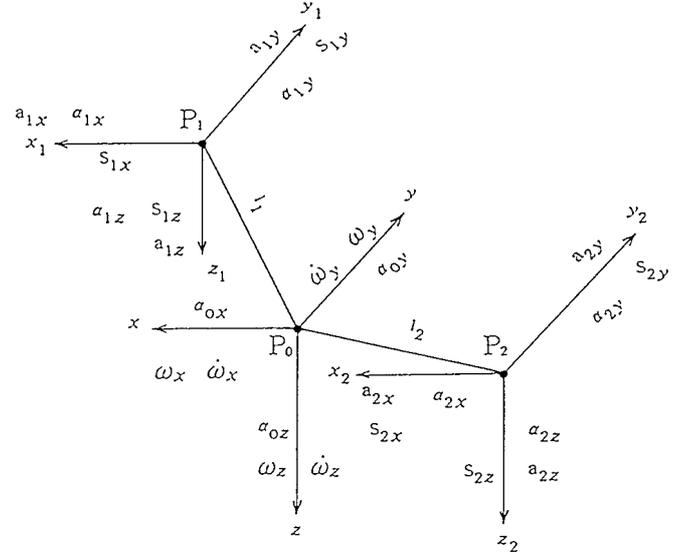
Fig.2 Inertial quantities in points  $P_0, P_1$  and  $P_2$
