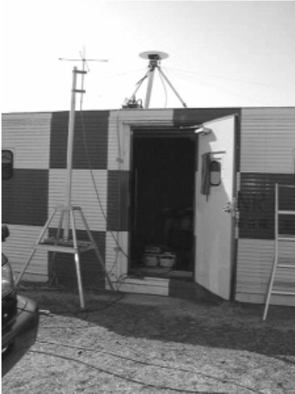
Figure 4-2 Ground monitor site, on which a Trimble Geodetic L1/L2 antenna was mounted, and the antenna of transmitter
