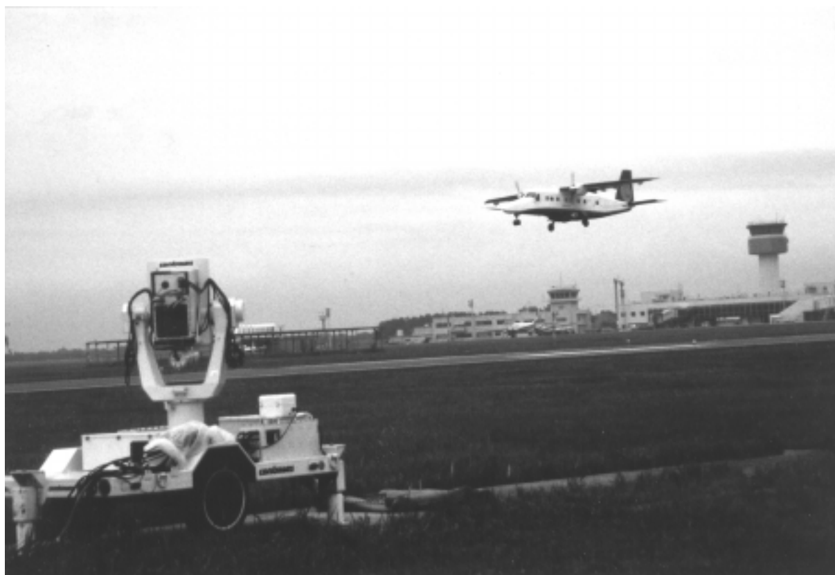
Figure 4-1 Research aircraft Do-228 and the laser tracker
