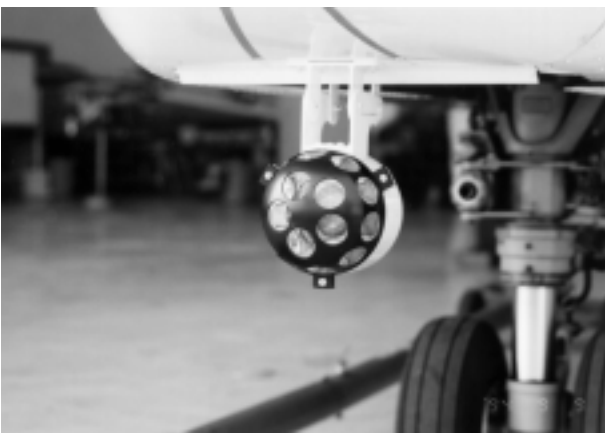
Figure 4-13 Laser reflector mounted under the nose of Do-228
