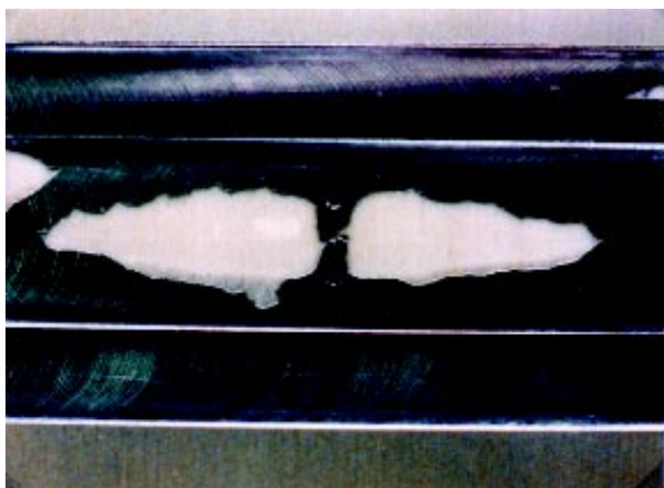
Fig. 14 Removal of the region swelling out of the plane in the GLARE3-5/4 at a 30mm under constant amplitude loading of \sigma_{max} = 147 MPa.
