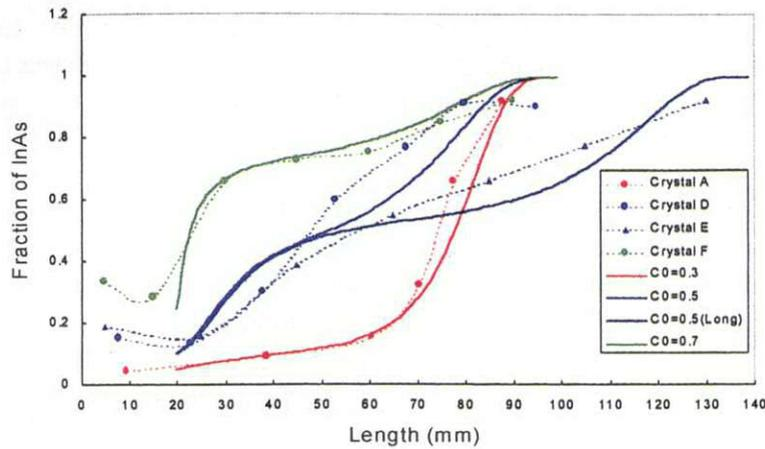
Fig.6 Comparison between the experimental and theoretical compositional profiles. Theoretical profiles with initial composition of 0.3 to 0.7 are calculated using the one dimensional diffusion model assuming the diffusion coefficient of  $6 \times 10^{-5} \text{cm}^2/\text{s}$ .
