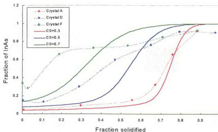
Fig.5 Compositional profiles along the growth direction versus fraction solidified. Solid lines are theoretical profiles with initial composition of 0.3 to 0.7 calculated assuming the normal freezing.
