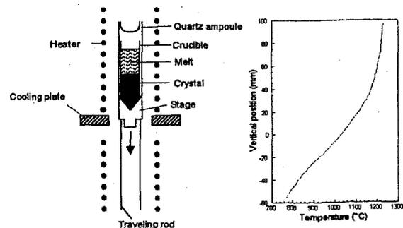
Fig.1 Schematic growth furnace and the temperature profile along the growth axis. A temperature gradient is 40 ~ 60° C/cm.
