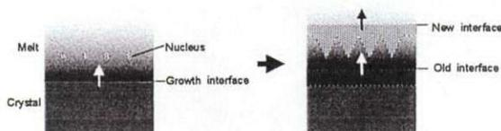
Fig.3 Schematic image of the phenomenon caused by the constitutional supercooling. Arrows at growth interfaces indicate the growth direction. Darker color represents higher InAs concentration.
