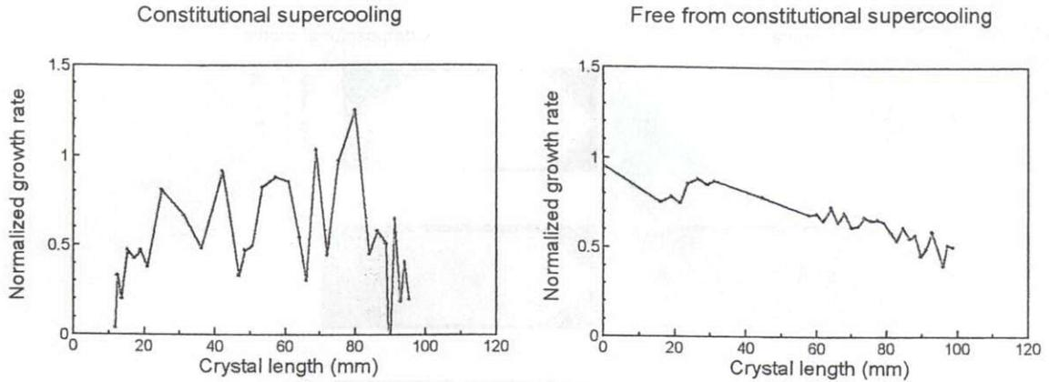
Fig.4 Variations of growth rates calculated from in-situ measured positions of growth interfaces. Growth rate is normalized by the travelling rate of the crucible.
