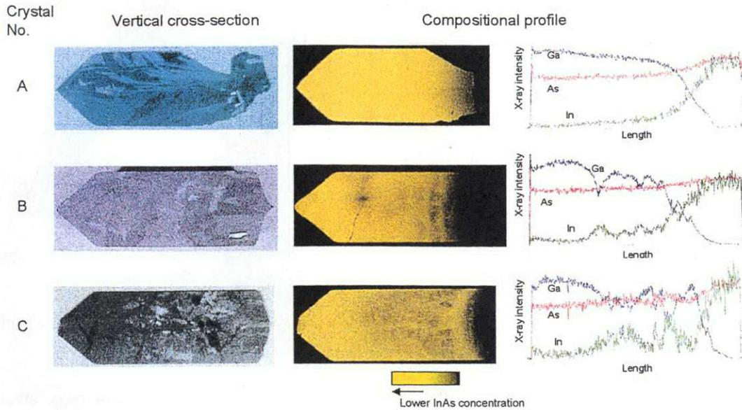
Fig.2 Photographs of vertical cross-sections and compositional profiles measured by the fluorescent X-ray method for crystal A~C. Compositional mappings are drawn by signal intensities of Ga-K  $\alpha$ . Graphs at the right sides are line distributions of X-ray intensities from each component at the center of crystals along the growth direction.
