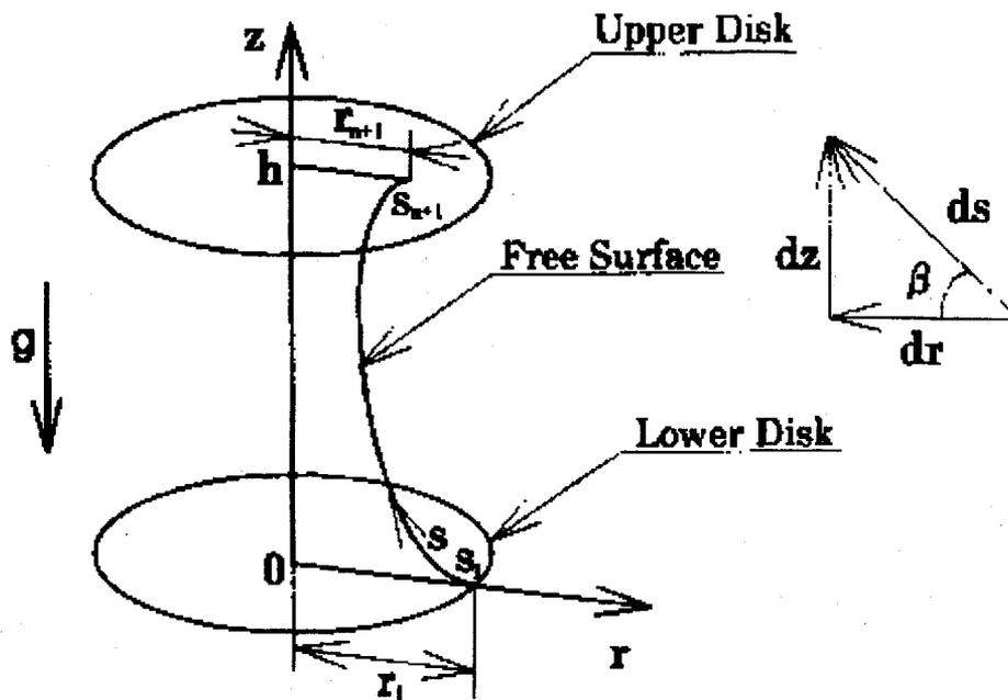
Figure 5-1. Calculation for meniscus of liquid bridge
