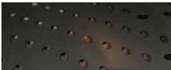
Figure 10: Porous wall of the S2MA test section.
