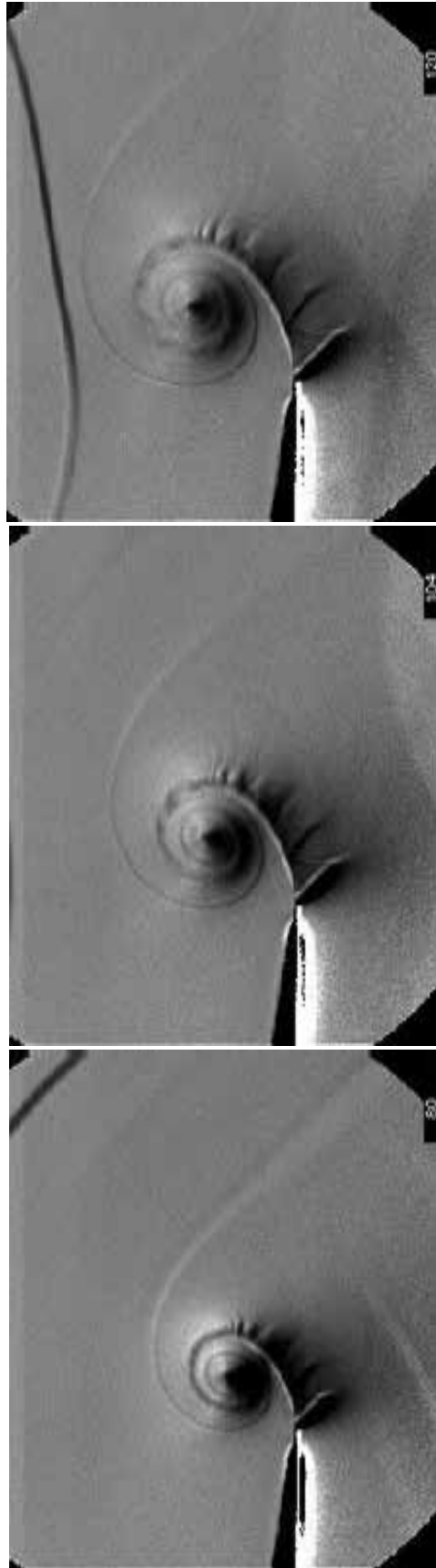
Figure 12. Schlieren montage of close-up images at 80, 104 and 120 \mu s after shock impingement
