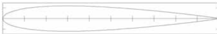
Figure 5: Airfoil section geometry (NACA 0012)
