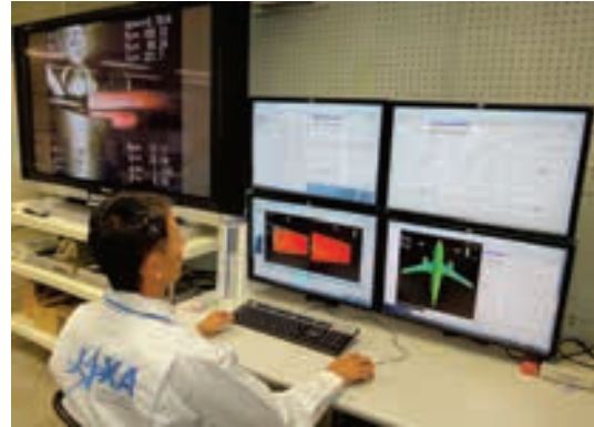
(b) Display setting for operation (balance, pressure sensor, PIV, PSP compared with CFD).
