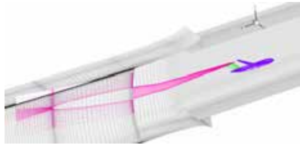
Figure 23: Mesh of the A310 research model in the S2MA test section.
