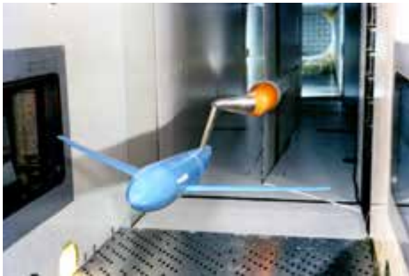
Figure 22: A310 model installed in the S2MA wind tunnel.
