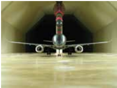
Ground effect test@ MHI 2m LWT
