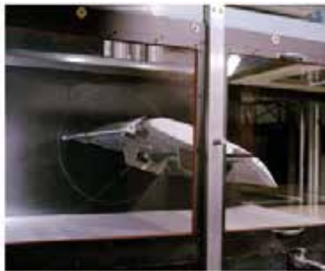
(a) 30P30N airfoil installed in the Basic Aerodynamics Research Tunnel [25]
