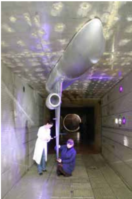
Figure 4. A half-model of a passenger aircraft in T-128 test section No 2
