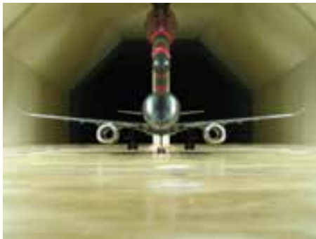
Ground effect test@ MHI 2m LWT
