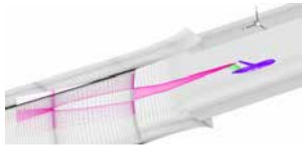
**Figure 23: Mesh of the A310 research model in the S2MA test section.**
