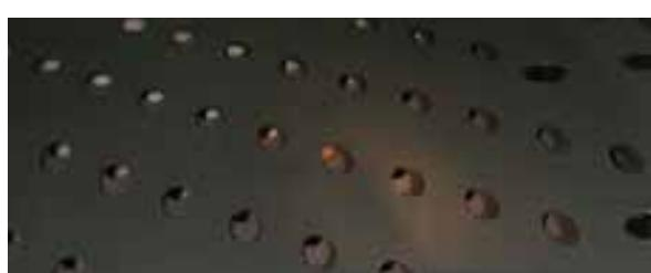
Figure 10: Porous wall of the S2MA test section.
