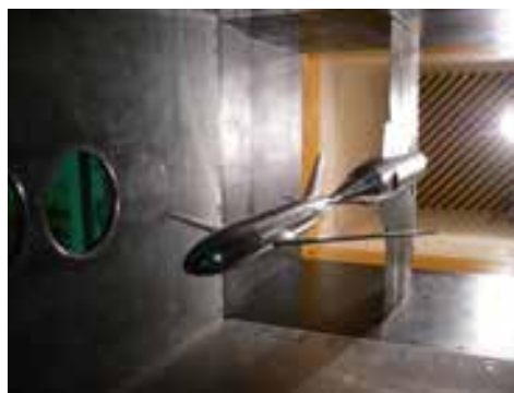
Figure 2 ONERA-M5 model installed in JTWT
