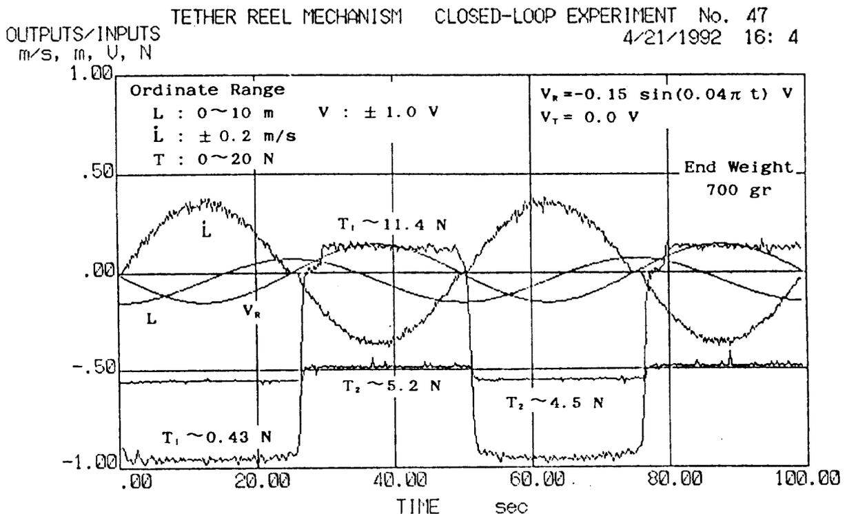
Fig. 14 Reel-Out/Reel-In with 0.02 Hz  $V_R$  and  $V_T = 0$
