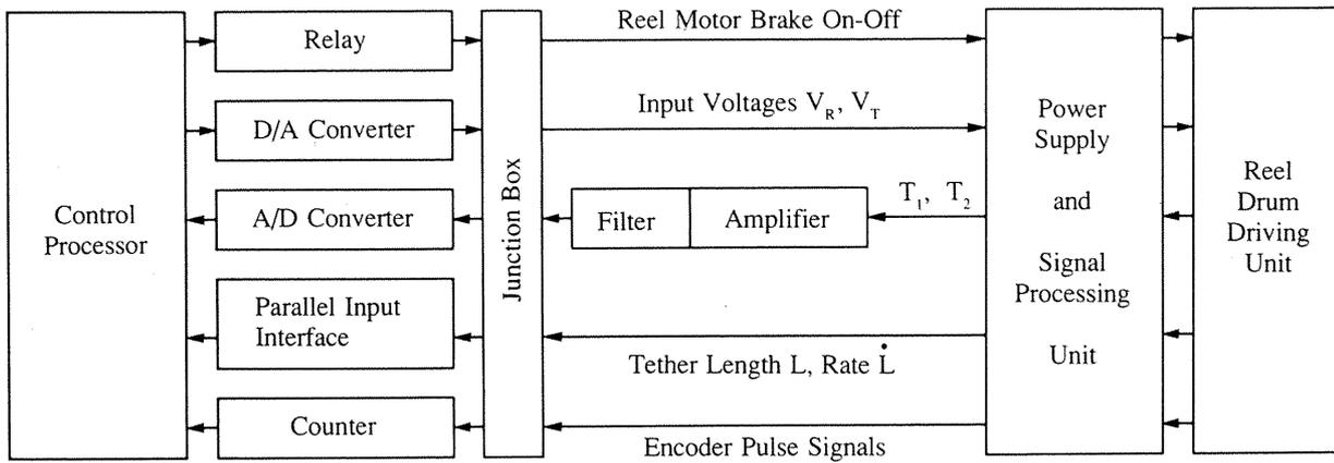
Fig. 8 Signal Flow of the Computer-Controlled Test System
