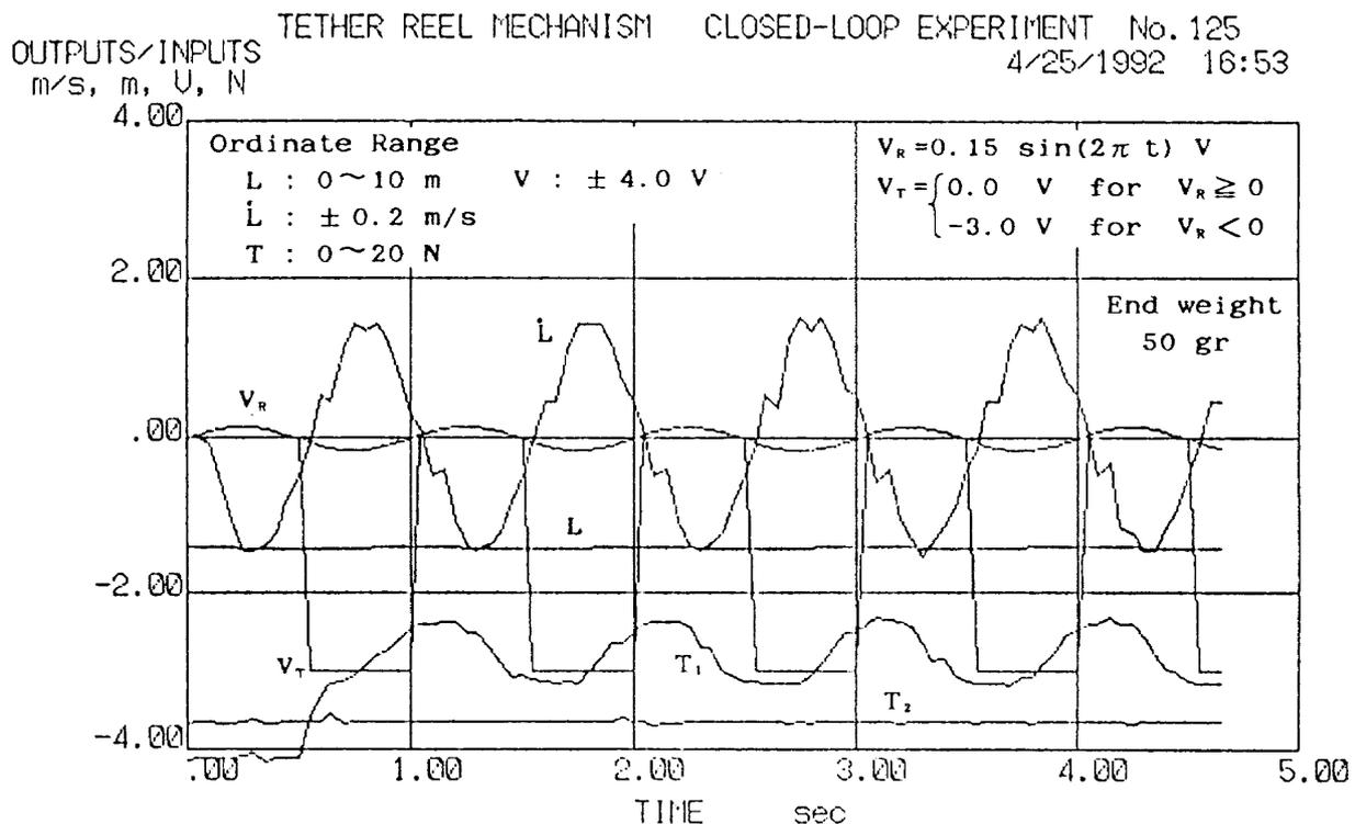
Fig. 19 Reel-Out/Reel-In with 1.0 Hz  $V_R$  and  $V_T = 0$  in 50 gr End Weight
