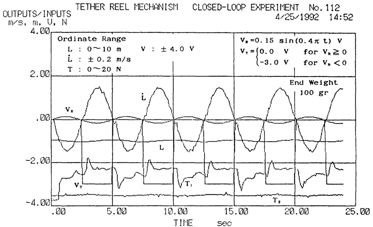
Fig. 18 Reel-Out/Reel-In with 0.2 Hz  $V_R$  and  $V_T = 0$  in 100 gr End Weight
