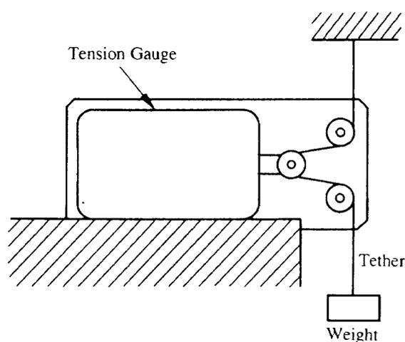
Fig. 7 Setup Configuration for Tension Gauge Calibration and Measuring Accuracy Test
