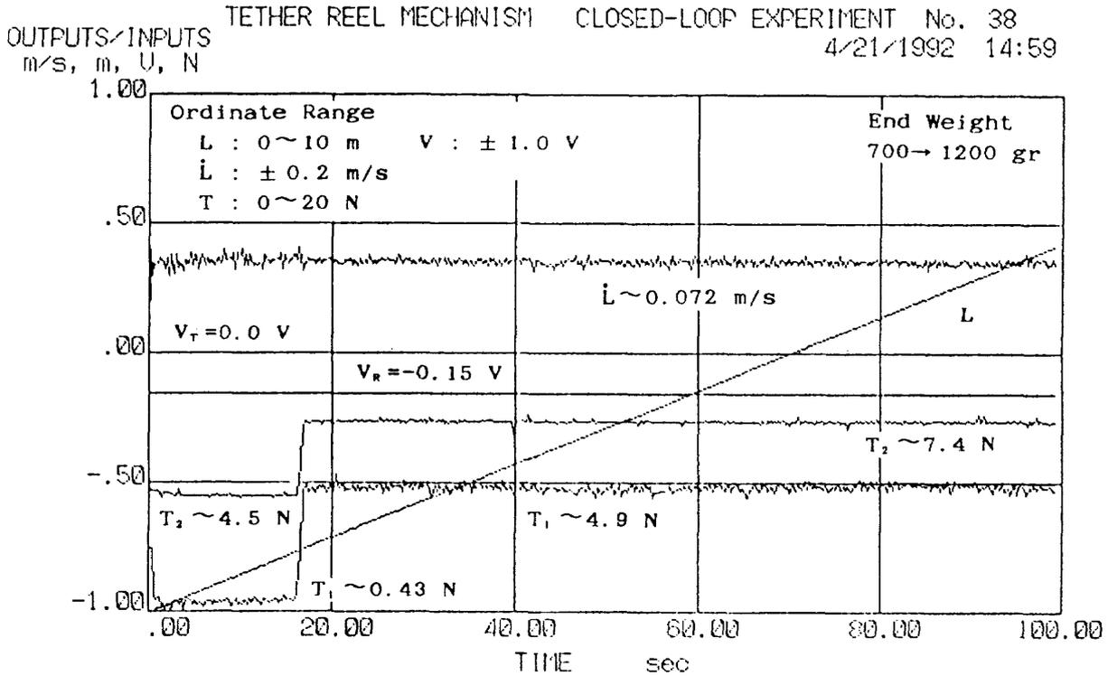
Fig. 12 Reel-Out Operation with Constant  $V_R$  and  $V_T = 0$
