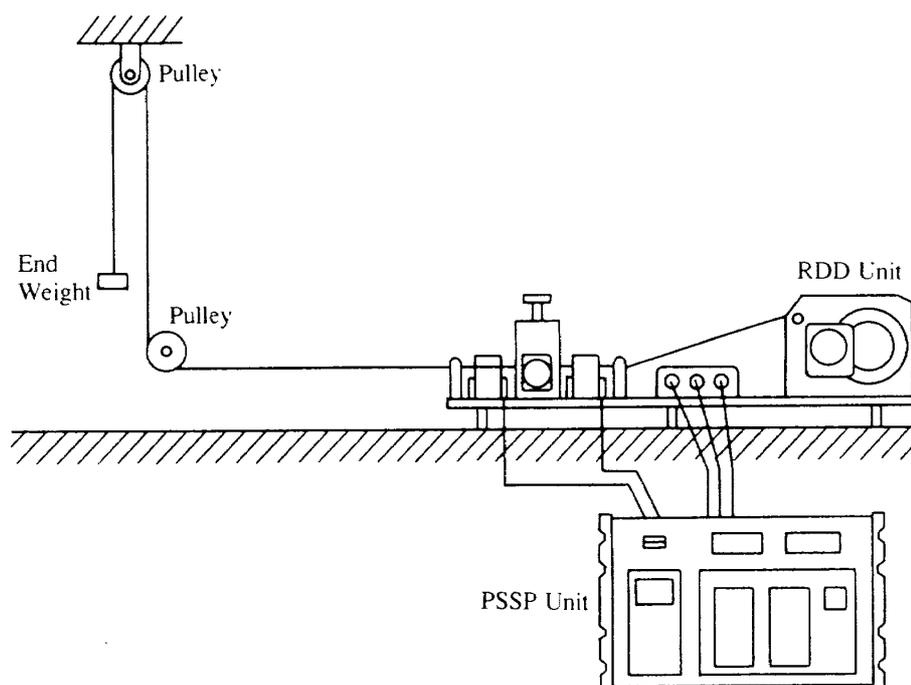
Fig. 6 Setup Configuration for Both Length/Rate Measuring Accuracy Test and Tension Adjusting Test
