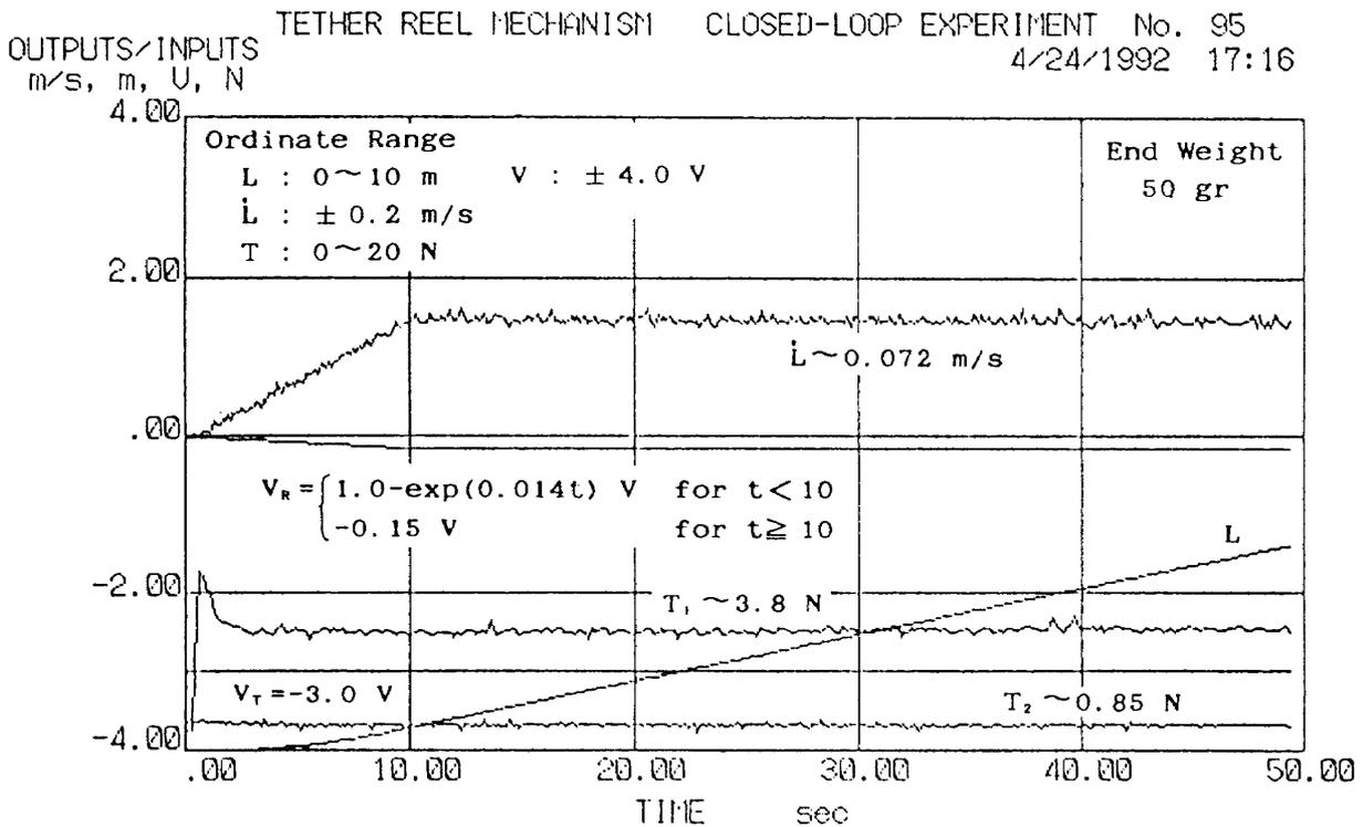
Fig. 16 Stable Reel-Out with  $V_T$  Input in 50 gr End Weight
