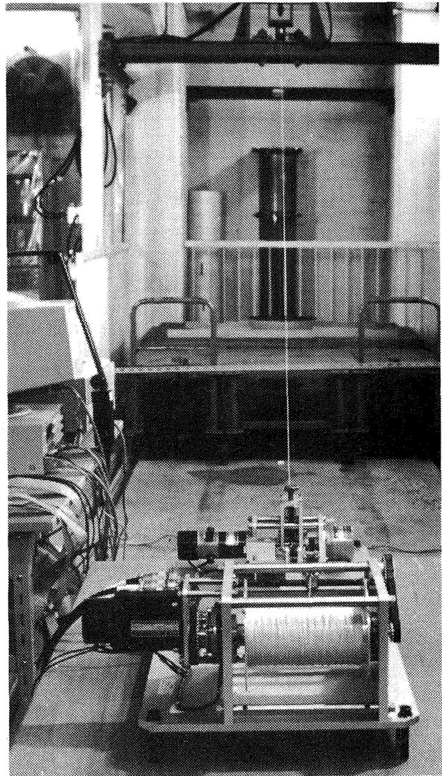
Fig. 11 Reel Drum Driving (RDD) Unit under Experiments in Drop Tower
