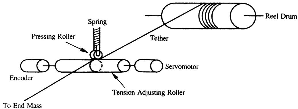
Fig. 3 Concept of Tension Adjusting Mechanism (TAM)
