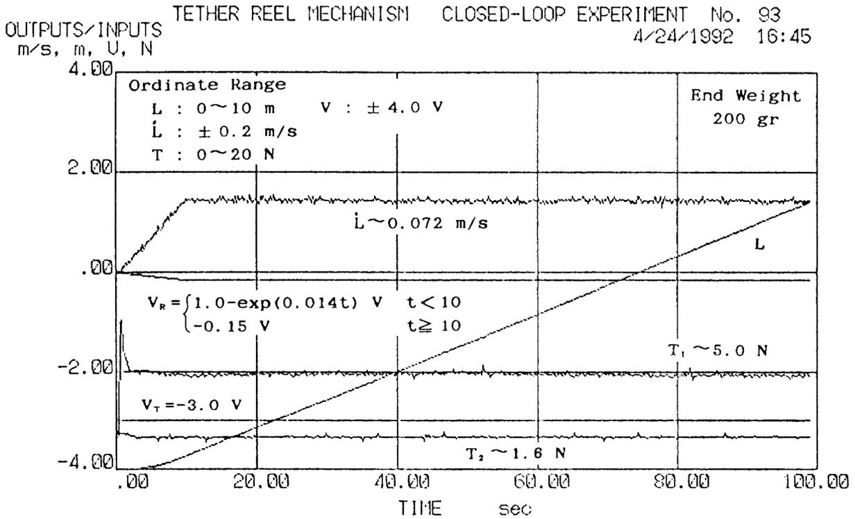
Fig. 15 Stable Reel-Out with  $V_T$  Input in 200 gr End Weight
