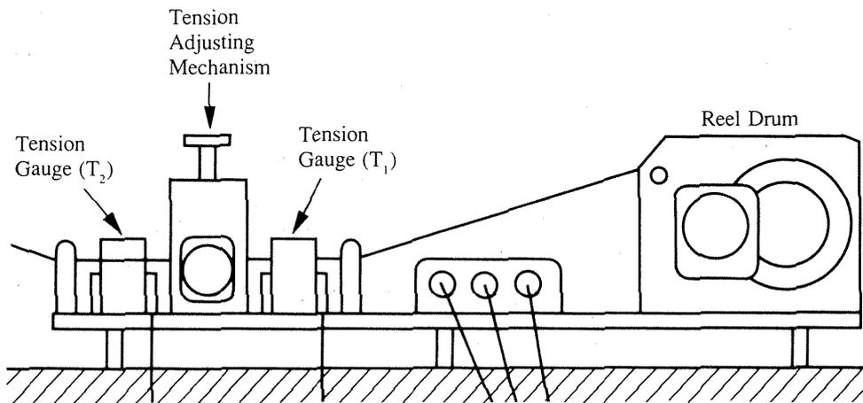
Fig. 2 Two Tension Gauges in Both Sides of TAM
