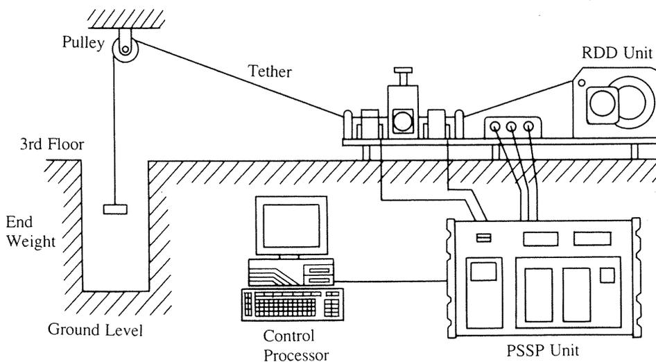
Fig. 10 Setup Configuration for the Computer-Controlled Test in Drop Tower
