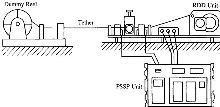
Fig. 5 Setup Configuration Including Dummy Reel for Preliminary Reel-out/Reel-in Test of Long Tether
