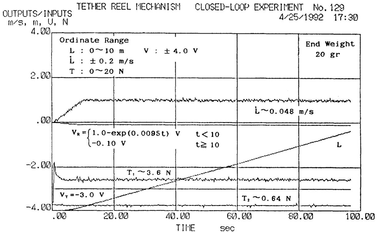
Fig. 17 Reel-Out by Smaller  $V_R$  Input with  $V_T$  Input in 20 gr End Weight
