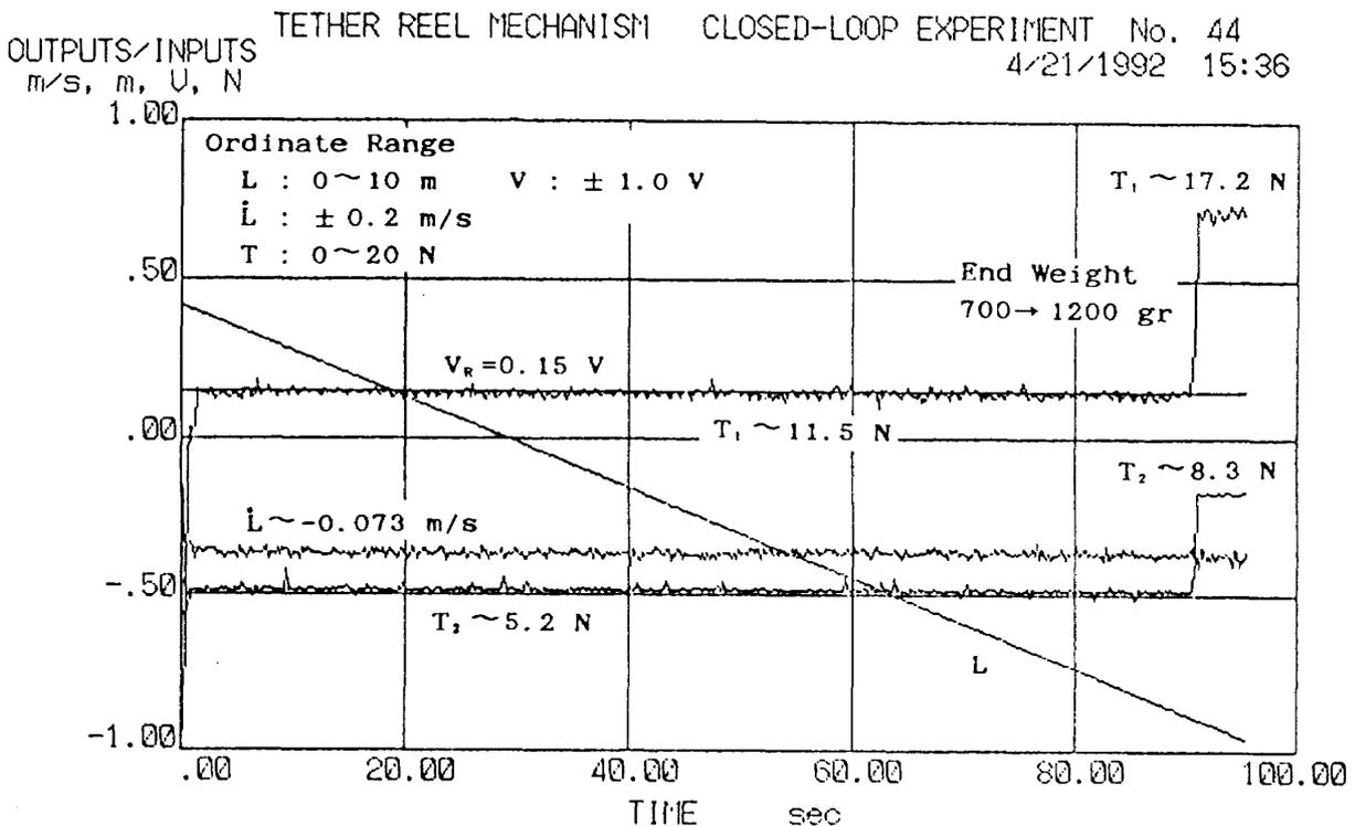
Fig. 13 Reel-In Operation with Constant  $V_R$  and  $V_T = 0$
