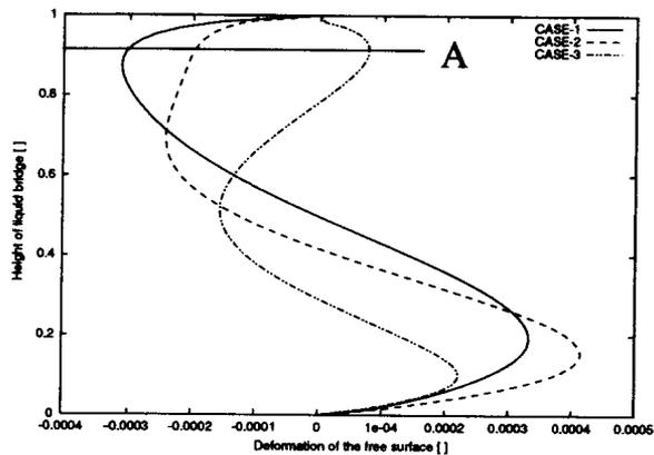
Figure 13: Free surface deformation in the steady state (CASE 1-3)
