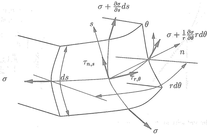
Figure 3: The stress balance between the shearing stress and the surface tension
