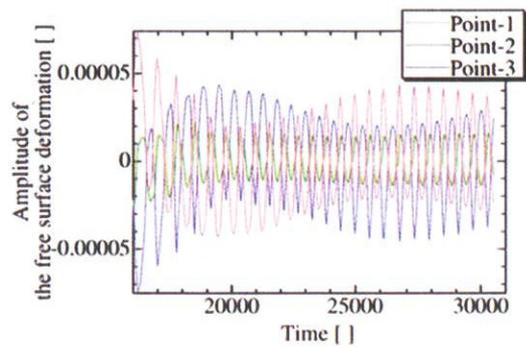
Figure 54: The oscillation amplitude of the free surface (CASE-8)
