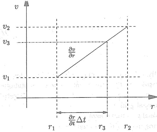
Figure 2: The relation between the velocity and the computational grid
