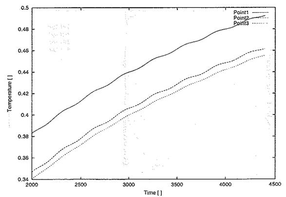
Figure 22: Variation of the free surface temperature (CASE-3)
