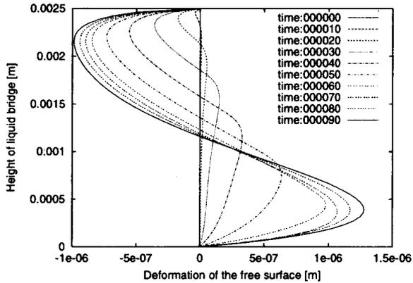
Figure 7: Displacement of the free surface deformation (CASE-1)
