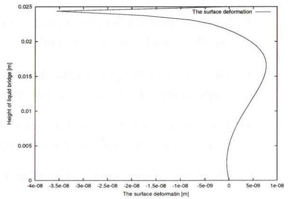
Figure 56: The free surface deformation of three dimensional analysis
