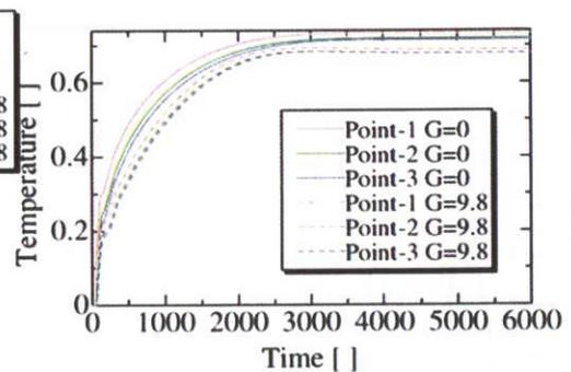
Figure 36: Variation of the free surface temperature (CASE-5 and 6)
