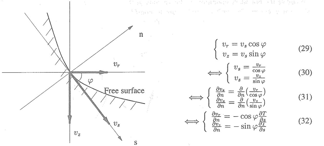
Figure 4: The velocity at the free surface
