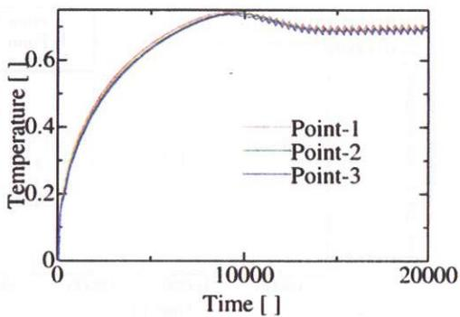
Figure 39: Variation of the free surface temperature (CASE-7)
