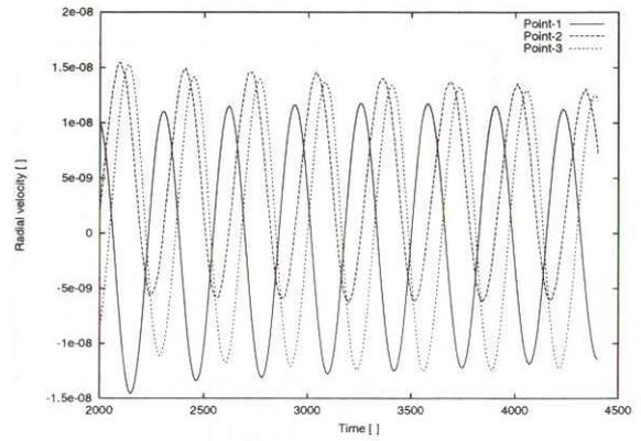
Figure 26: Variation of the radial velocity on the free surface in CASE-3  $\times 10^{-3}$
