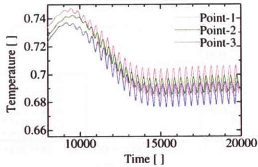
Figure 43: Variation of the free surface temperature (CASE-7)
