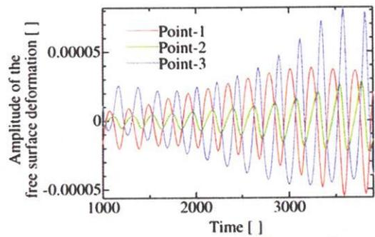
Figure 34: The oscillation amplitude of the free surface in CASE-4
