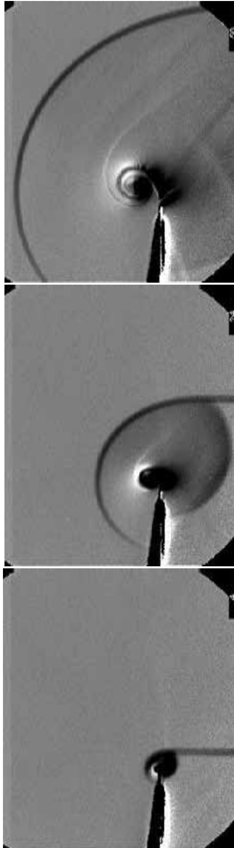
Figure 10. Schlieren montage of close-up images at 4, 24 and 56 \mu\text{s} after shock impingement
