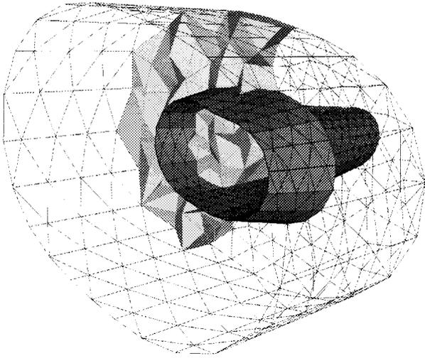
Fig. 6: General view of the computational domain. A cowl and an outer part are attached to the inlet shown in Fig. 5. The latter is to accommodate a bow shock in case the inlet unstarts. Surface mesh on some boundaries of the computational domain and some part of the internal tetrahedra are shown; the inlet's and cowl's surfaces and tetrahedra are shaded.
