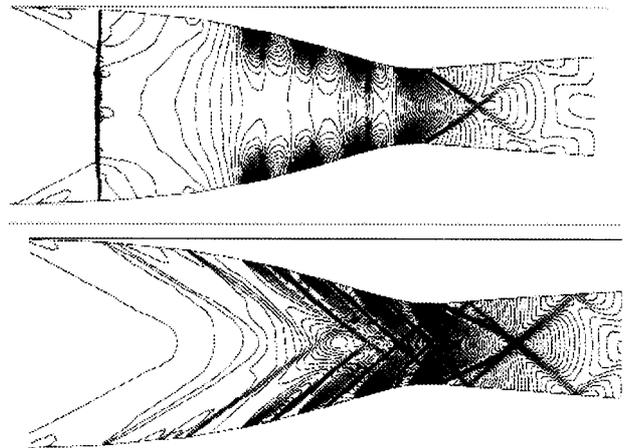
Fig. 3: An example of successful inlet starting using perforations. Top: a part of the bow shock (see Fig. 2) has entered the converging portion of the duct. Bottom: the shock has moved completely past the throat and flow through the inlet is fully supersonic. Density contours are shown.
