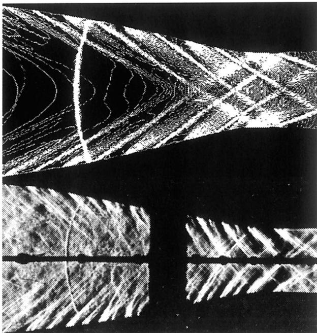
Fig. 4: Bottom: schlieren photograph of flow in the experimental inlet from [6] at Mach 2.5; double exposure shows starting shock and subsequent started flow. Top: 2-D CFD simulation of flow for the same configuration and similar conditions, showing constant density contours.
