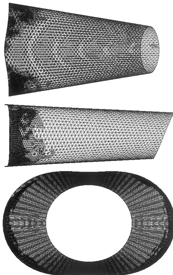
Fig. 5: A simplified three-dimensional nozzle under consideration; top, side and axis views are shown (from top to bottom); the images are not to scale.
