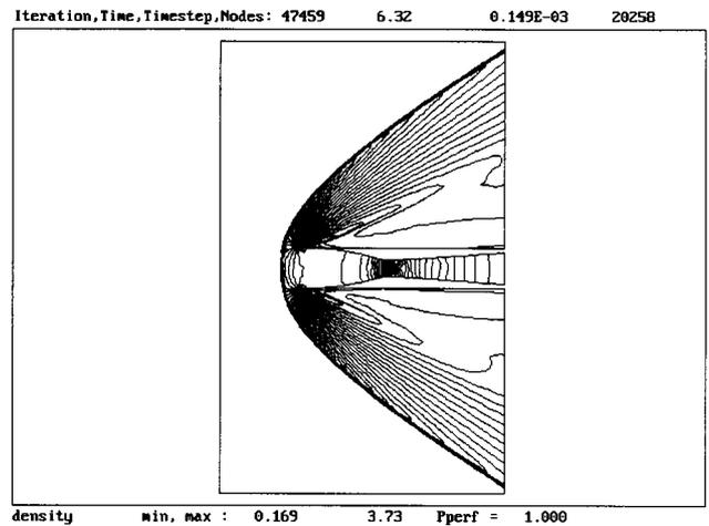
Fig. 2: The initial unstart state of the supersonic inlet at Mach 2.5 with the bow shock standing in front of the inlet's entrance (density contours).
