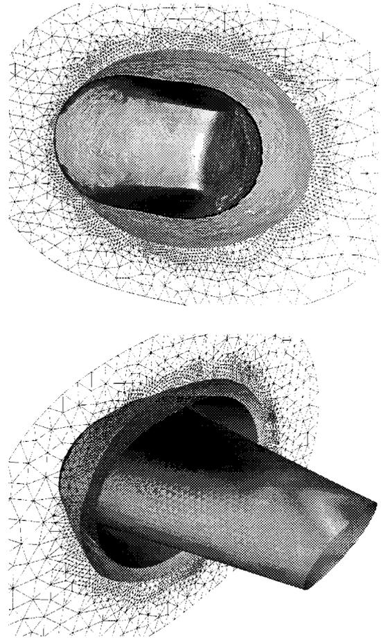
Fig. 7: The inlet starts at the freestream Mach number  $M = 4$ . The flow pattern to be eventually established is shown here from two different viewpoints. A pressure isosurface approximately represents the oblique shock wave attached to the cowl and a shock wave system inside the inlet. The inlet surface is colored according to pressure values.
