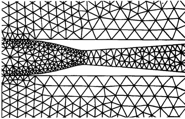
Fig. 1: The geometry of the two-dimensional inlet employed in this study and the background unstructured grid to be adaptively refined in the course of flow development.
