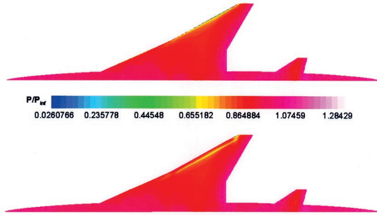
Fig.6 Upper surface pressure contours of initial (up) and LE flap design (down) shapes
