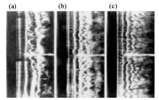
Fig. 5 Vortex tubes for the symmetric excitation at (a)  $u_f/U_\theta = \pm 0.05$ , (b)  $u_f/U_\theta = \pm 0.08$  and (c)  $u_f/U_\theta = \pm 0.10$ .
