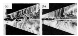
Fig. 3 Entrainment for (a)the antisymmetric excitation at  $u_f/U_\theta = \pm 0.05$  and (b)the symmetric excitation at  $u_f/U_\theta = \pm 0.10$ .
