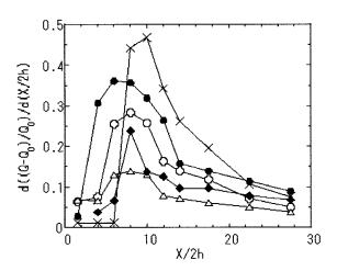
Fig. 4 Streamwise evolution of the entrainment rate. Natural jet;  $\times$ Antisymmetric excitation;  $\bullet: u_f/U_0 = \pm 0.05$ Symmetric excitation;  $\bigcirc: u_f/U_0 = \pm 0.05$ ,  $\bullet: \pm 0.08$   $\triangle: \pm 0.10$
