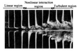
Fig. 2 Vortex arrangement for the symmetric excitation at  $u_f/U_0 = \pm 0.08$
