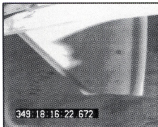
Figure 10. In-Flight infrared image of test wing showing extensive laminar flow.
