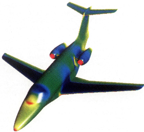
Figure 4: Typical business jet configuration. FLO107-MB: Navier-Stokes, Baldwin-Lomax, M = 0.80 , Re = 2.5 million, 5.8. million mesh cells. C_p contours.
