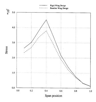
Figure 10: Spanwise Stress Distribution for the Rear Spar. Comparison of the Rigid Design and the Baseline Design. Wing Alone Configuration. Rigid Design, Drag Minimization at Fixed  $C_L$ . Aeroelastic Analysis at Fixed  $C_L$ .
