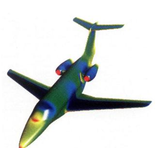
Figure 4: Typical business jet configuration. FLO107-MB: Navier-Stokes, Baldwin-Lomax,  $M=0.80,\,Re=2.5\,$  million, 5.8. million mesh cells.  $C_p$  contours.
