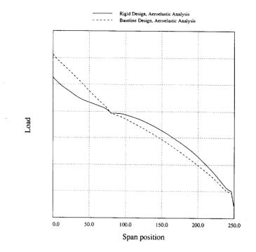
Figure 9: Spanwise Load Distribution. Comparison of the Rigid Design and the Baseline Design. Wing Alone Configuration. Rigid Design, Drag Minimization at Fixed  $C_L$ . Aeroelastic Analysis at Fixed  $C_L$ .
