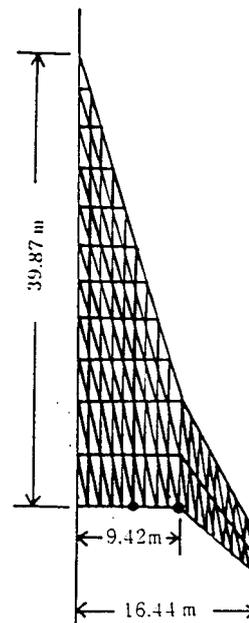
Fig. 2 Finite Element Grid
