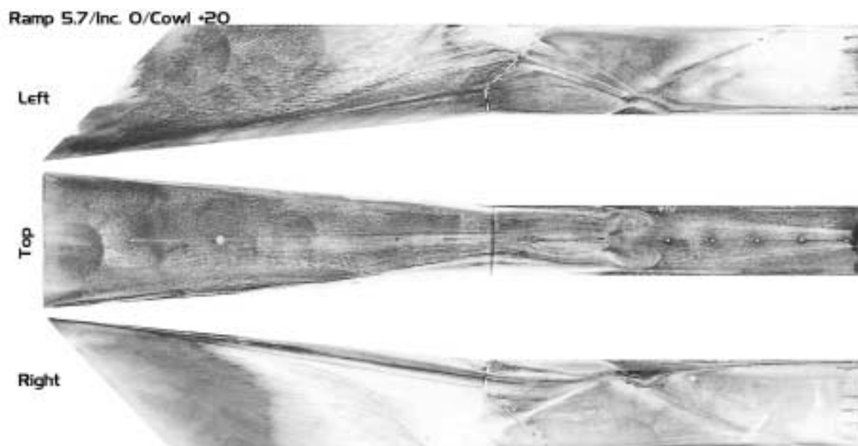
Fig. A-1 Oil flow pattern of the extended-cowl model (ramp model \alpha = 5.7^\circ , inclination \delta = 0^\circ ).
