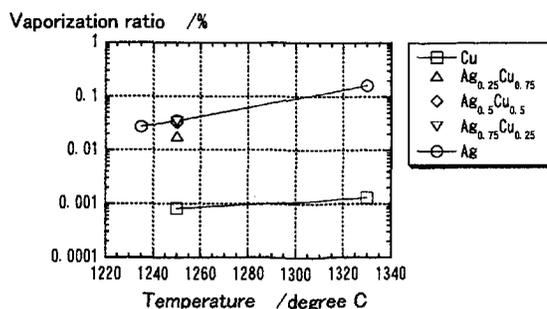
**Figure 5 Calculated vaporization ratio for the diffusion experiments**
