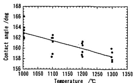
**Figure 3 Contact angle between boron nitride and Ag<sub>0.5</sub>Cu<sub>0.5</sub>**
