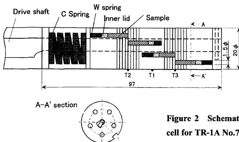
Figure 2 Schematic drawing of the shear cell for TR-1A No.7 rocket experiments
