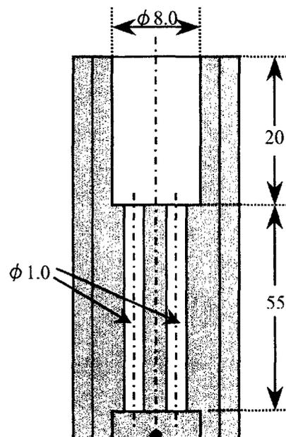
**Figure 2 Crucible for casting a cylindrical sample with 1.0 mm diameter**
