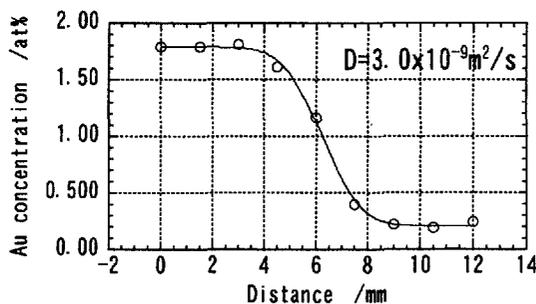
**Figure 3** Concentration distribution after the diffusion experiment at 1273 K
