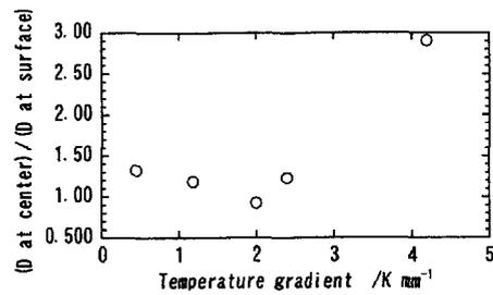
Figure 5 Normalized diffusion coefficient vs. temperature gradient
