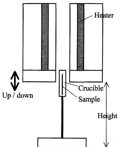
**Figure 3 Configuration of the sample and the furnace**
