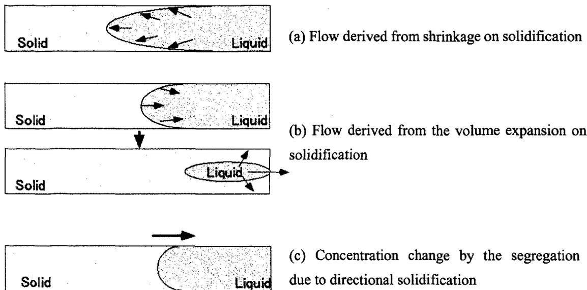
**Figure 1 Schematic figures of solidification effects on diffusion experiments**
