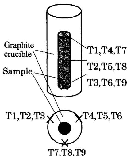
**Figure2 Position of the thermocouples put on a crucible**
