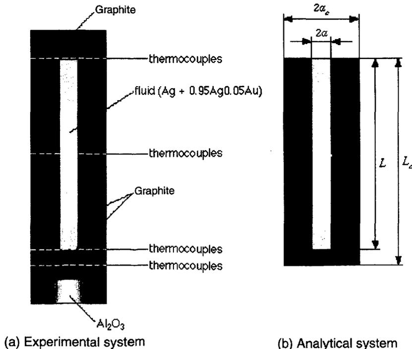
Fig.1 Experimental system and analytical system of this study
