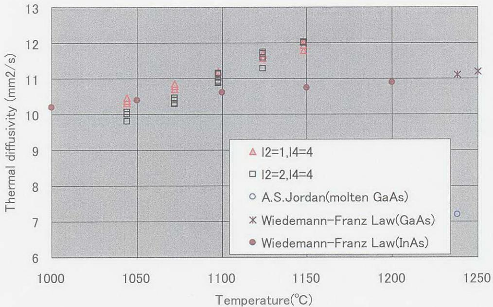
Fig. 5 Thermal diffusivity of molten In<sub>0.8</sub>Ga<sub>0.2</sub>As
