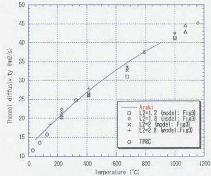
Fig. 4 Thermal diffusivity of molten Ga
