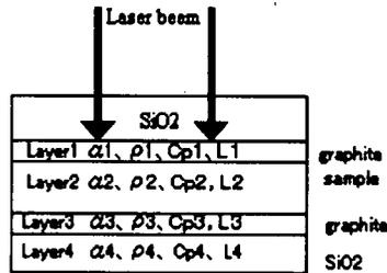
Fig.3 Model of a specimen
