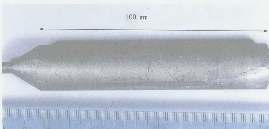
Fig.5 Shaped \text{In}_x\text{Ga}_{1-x}\text{As} source material having a graded concentration
