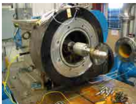
2-blade inducer with on-rotor dynamic force measurement system
