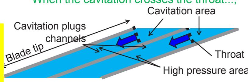
Cavitation plugs channels between blades because cavitation bubbles are **big**. Therefore, **the pump does not work**.
