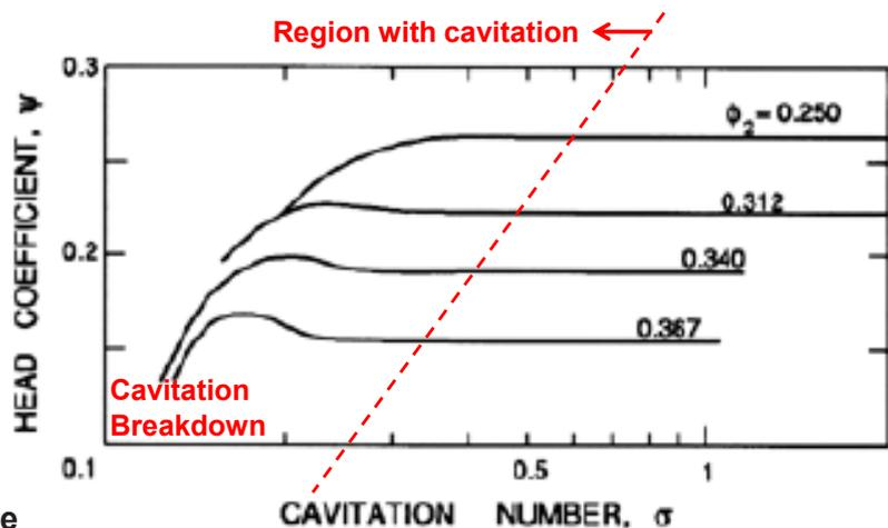
Establishment of a **Design Method for Cryogenic Inducer Allowing Cavitation**
