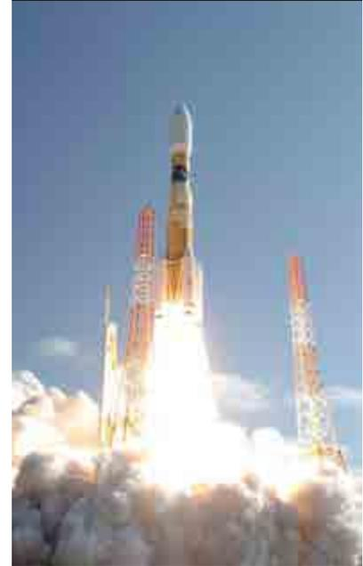
Launch rocket **without solid rocket boosters** is ideal for manned mission. To do this, **reliable liquid rocket engines with sufficient thrust** are required !!
