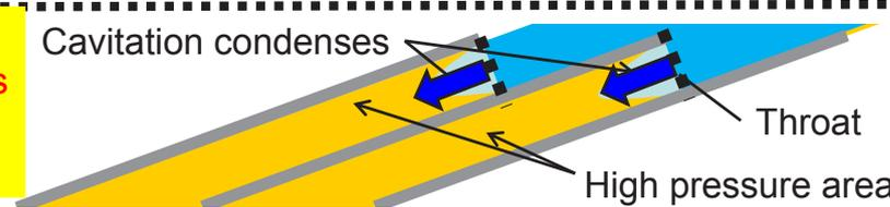
Cavitation condenses between blades because cavitation bubbles are **small**. Therefore, **the pump works**.
