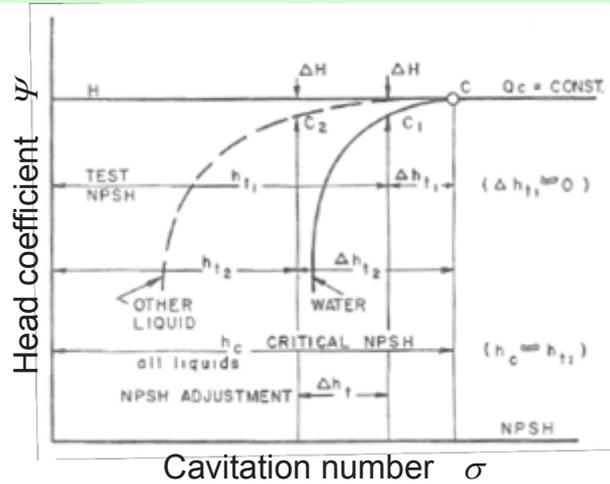
**Therefore, it is well known that fluid with greater thermodynamic effect is less subject to cavitation breakdown.**
