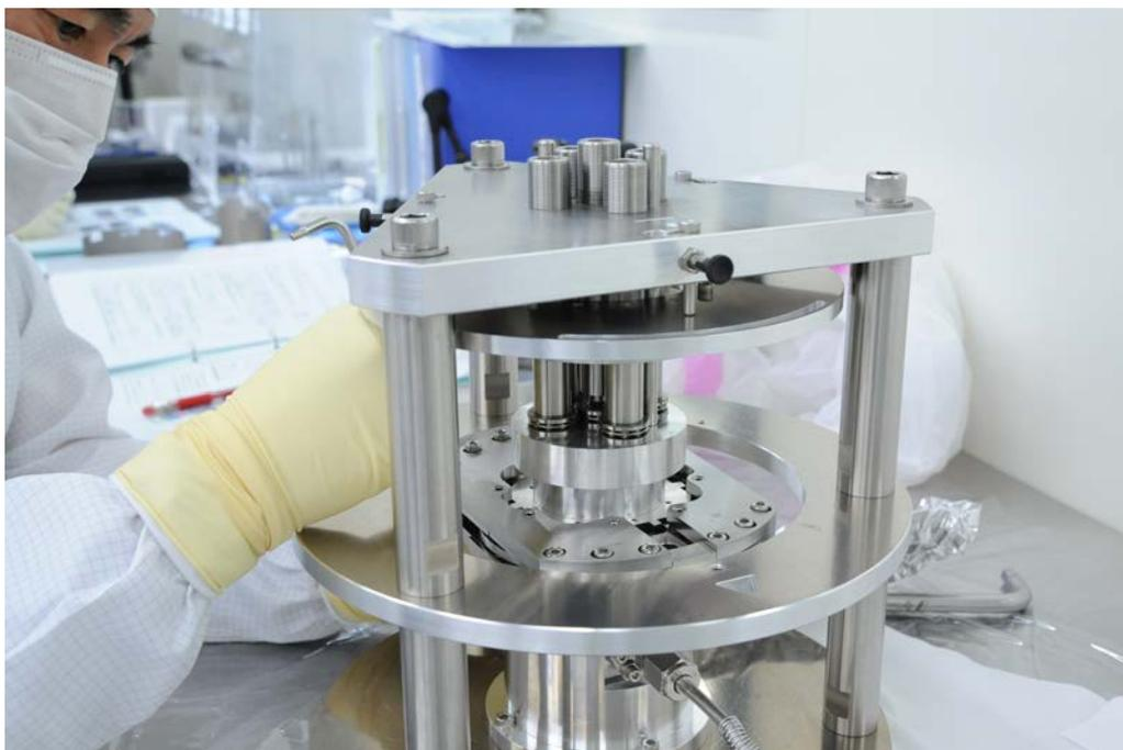
Fig. 15. A snapshot of a rehearsal for removal of the outer lid, the frame for latches and NEA from the sample container. The simulated container equips a vacuum flange, though which we could check the condition inside the container.
