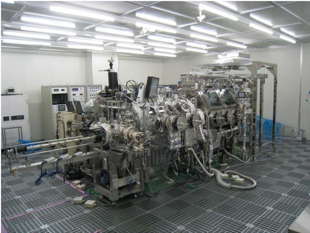
Fig. 2. A photograph of clean chambers in the Planetary Material Sample Curation Facility (PMSCF) of JAXA. They consist of two main chambers, No.1 (left) and No.2 (right) and situate in the planetary sample handling room of 100 – 1,000 in clean class level of Fed. Std. 209D.
